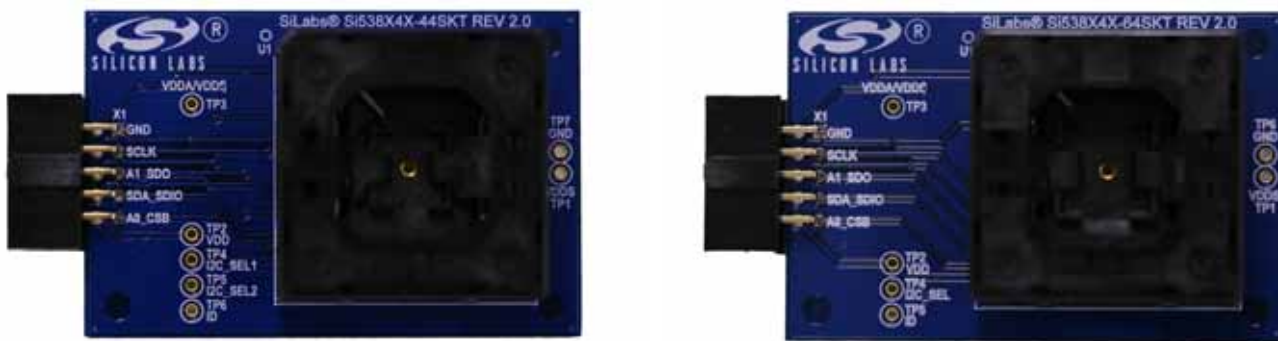
Figure 4. Si538x4x-44SKT-DK (l) and Si538x4x-64SKT-DK (r) Sockets Sold Separately
