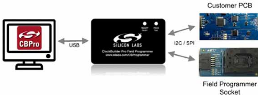
Figure 5. PC to CBPROG-DONGLE Connection
