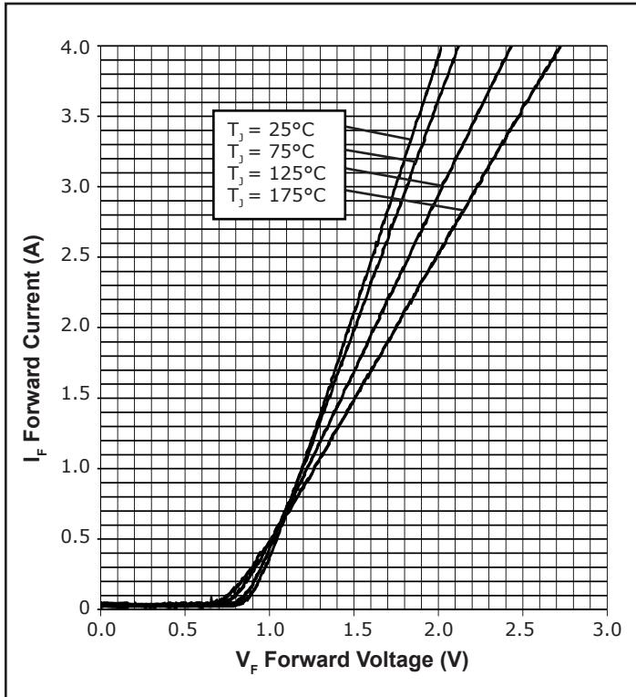
Figure 1. Forward Characteristics
