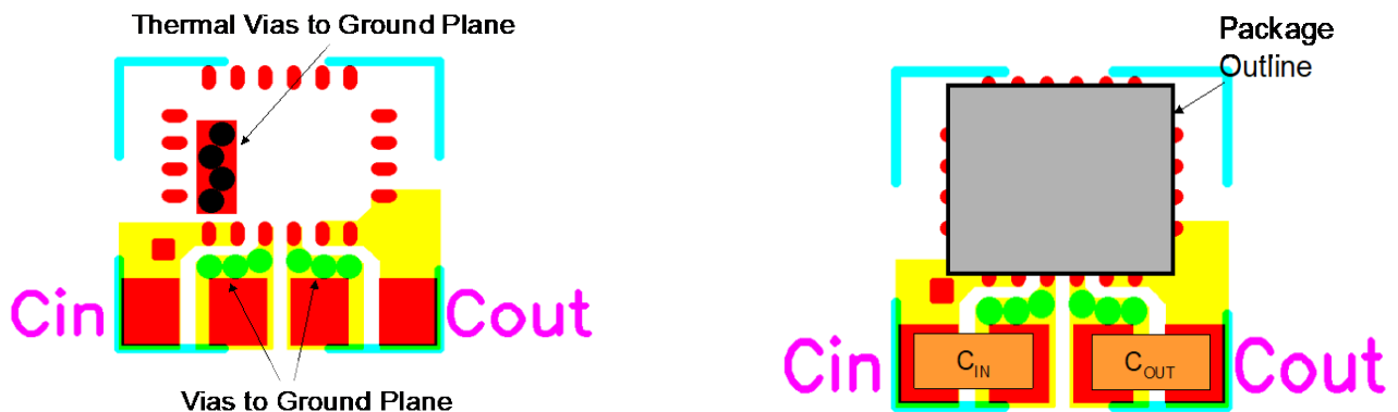
Figure 8. Example layout showing PCB top layer, as well as demonstrating use of vias from input, output filter capacitor local grounds, and thermal pad, to PCB system ground
