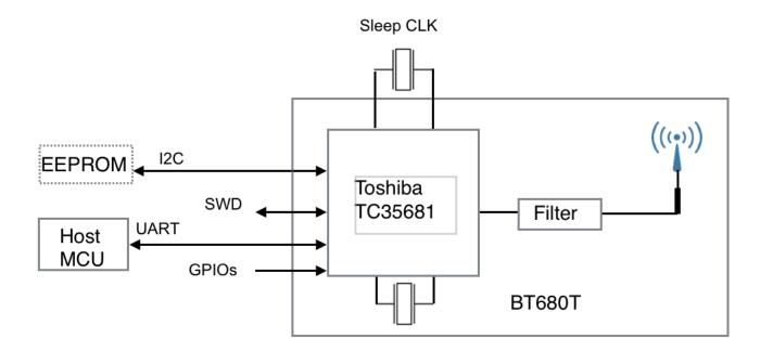
Sister module BT680TA is identical to BT680T except automobile temperature components are used.
