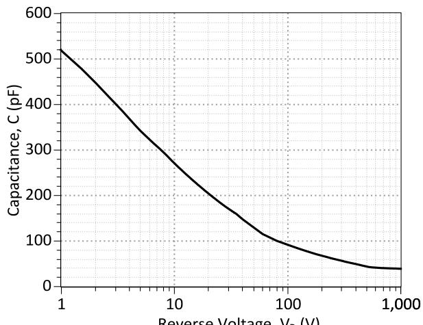
Figure 5: Typical Junction Capacitance vs Reverse Voltage Characteristics
