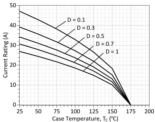
Figure 4: Current Derating Curves ( $D = t_p/T$ ,  $t_p = 400 \mu s$ )
