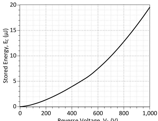
Figure 6: Typical Switching Energy vs Reverse Voltage Characteristics
