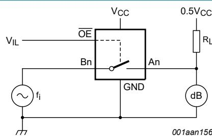
Adjust  $f_i$  voltage to obtain 0 dBm level at output. Increase  $f_i$  frequency until dB meter reads -3 dB.**Fig. 17. Test circuit for measuring the frequency response when channel is in ON-state**
