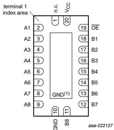
(1) This is not a ground pin. There is no electrical or mechanical requirement to solder the pad. In case soldered, the solder land should remain floating or connected to GND.
