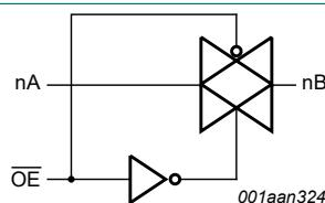
Fig. 2. Logic diagram (one switch)
