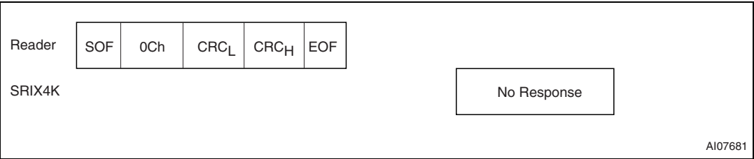
Figure 41. Reset_to_inventory frame exchange between reader and SRIX4K
