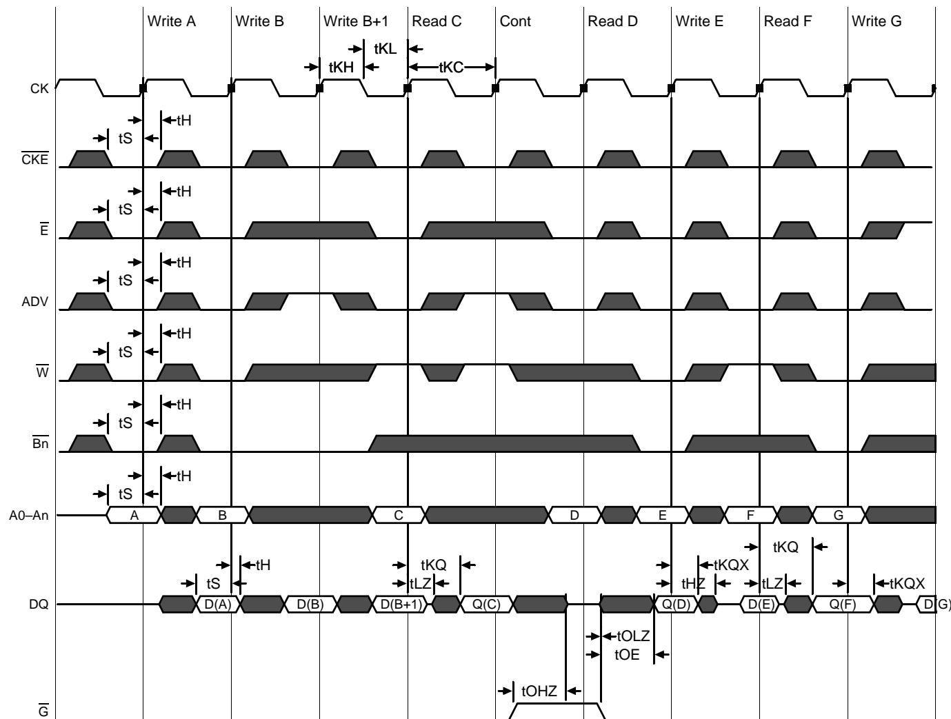
\*Note:  $\bar{E} = \text{High}(\text{False})$  if  $\bar{E}_1 = 1$  or  $E_2 = 0$  or  $\bar{E}_3 = 1$
