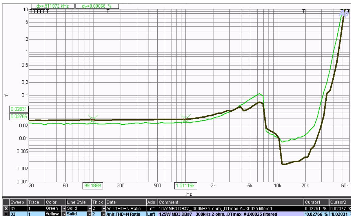
Figure 4 THD+N vs. Frequency at 10W and 125W
