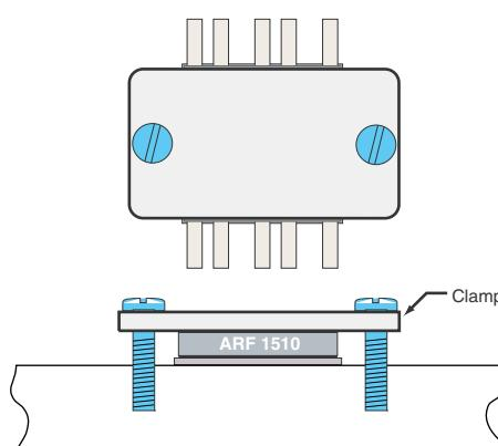
The package is designed to be clamped to a heatsink. A clamped joint maintains the required mounting pressure while allowing for thermal expansion of both the device and the heat sink. A simple clamp, and two 6-32 (M3.5) screws can provide the minimum 125 lb. required mounting force. T=4-6 in-lb. Please refer to App Note 1802 "Mounting Instructions for Flangeless Packages."
