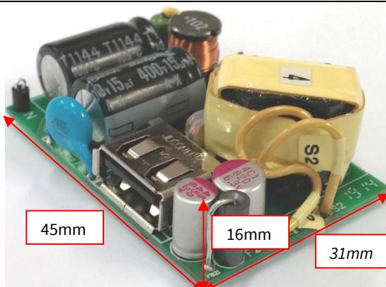
**Figure 1** REF-15W\_CE1K5 ADAPTER [Dimensions L x W x H: 45mm x 31mm x 16mm]
