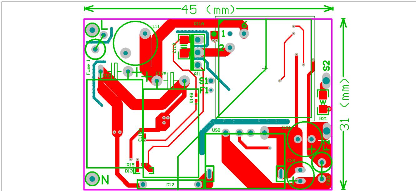
**Figure 4** Top side copper and component legend
