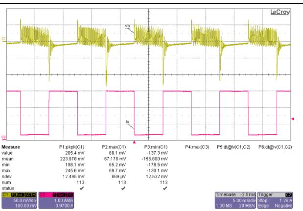
Channel 1; C1 : Output ripple voltage ( $V_{\text{out}}$ )
