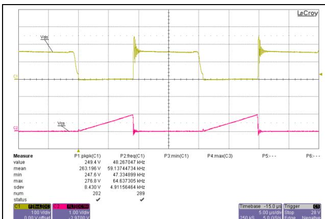
Channel 1; C1 : Drain-source voltage ( $V_{\text{DS}}$ )
