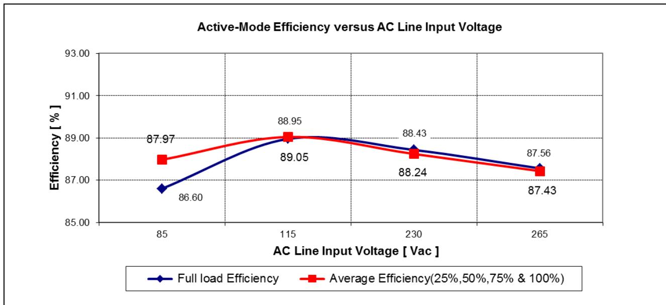
**Figure 7 Efficiency vs AC line input voltage**
