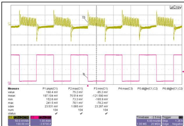
Channel 1; C1 : Output ripple voltage ( $V_{\text{out}}$ )
