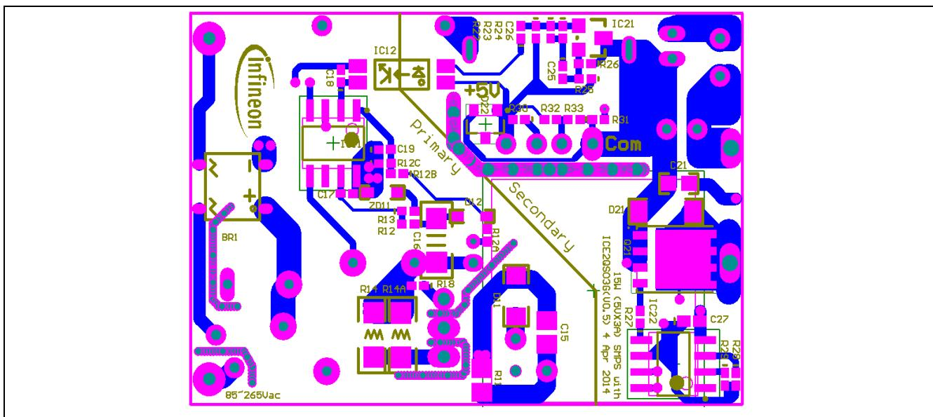
**Figure 5** Bottom side copper and component legend
