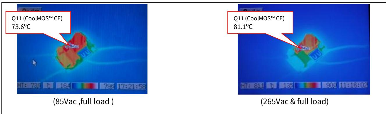
**Figure 17 Infrared thermal image of REF-15W\_CE1K5 ADAPTER**
