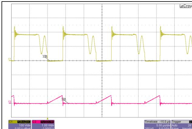
Channel 1; C1 : Drain voltage ( $V_{\text{Drain}}$ )
