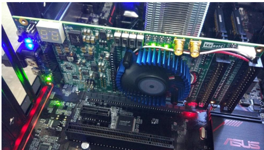
Figure 7-8 FPGA board installation on PC
