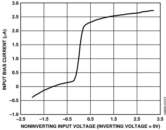
Figure 8. Input Bias Current vs. Input Voltage
