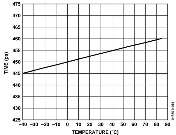
Figure 13. Fall Time vs. Temperature
