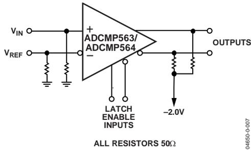
Figure 24. High Speed Sampling Circuits
