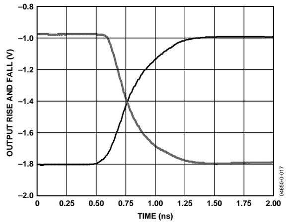
Figure 12. Rise and Fall of Outputs vs. Time
