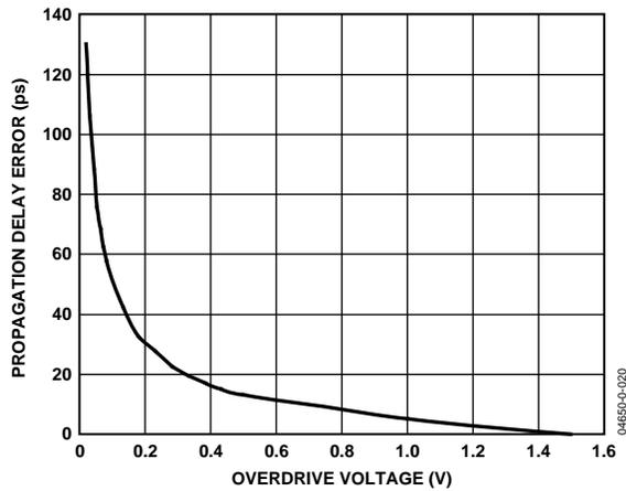
Figure 15. Propagation Delay Error vs. Overdrive Voltage
