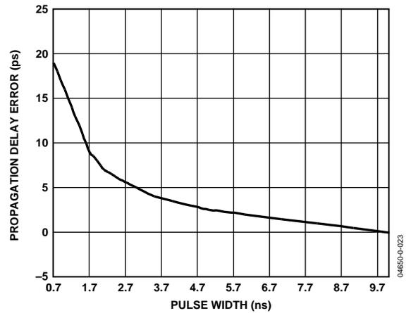
Figure 18. Propagation Delay Error vs. Pulse Width
