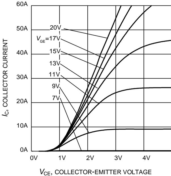
**Figure 5. Typical output characteristic**
