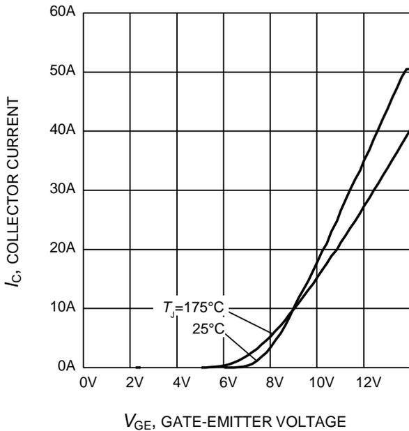
**Figure 7. Typical transfer characteristic**
