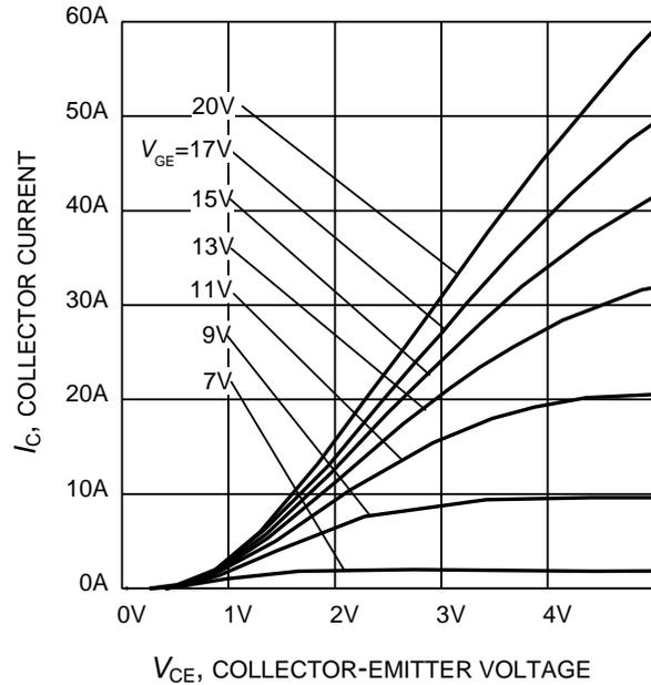
**Figure 6. Typical output characteristic**
