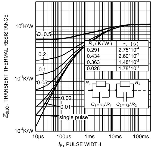
**Figure 24. Diode transient thermal impedance as a function of pulse width**
