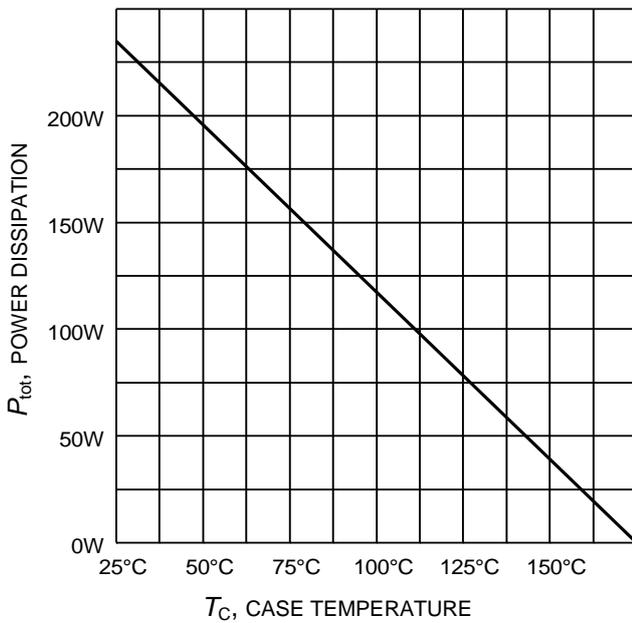
**Figure 3. Maximum power dissipation as a function of case temperature**
