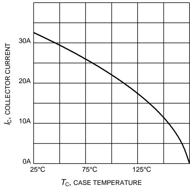
**Figure 4. Maximum DC Collector current as a function of case temperature**
