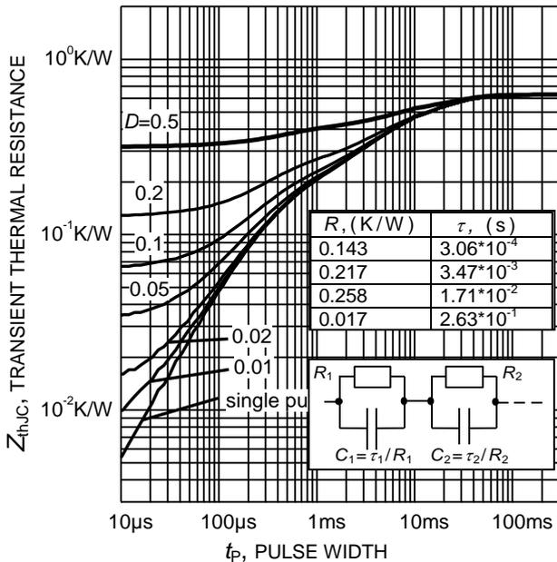
**Figure 23. IGBT transient thermal resistance**
