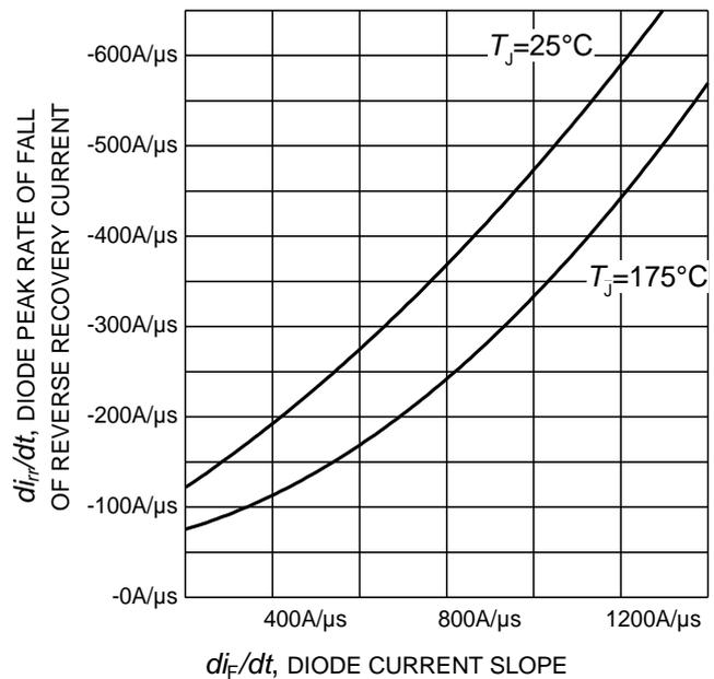
**Figure 26. Typical diode peak rate of fall of reverse recovery current as a function of diode current slope**
