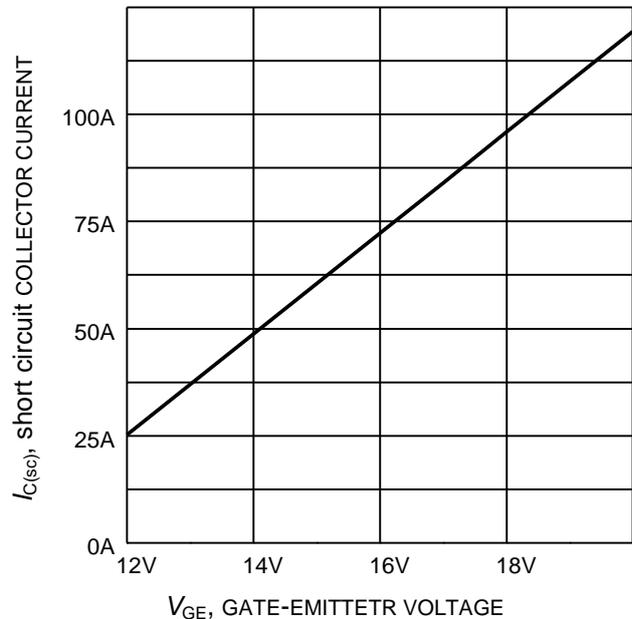
**Figure 20. Typical short circuit collector current as a function of gate-emitter voltage**
