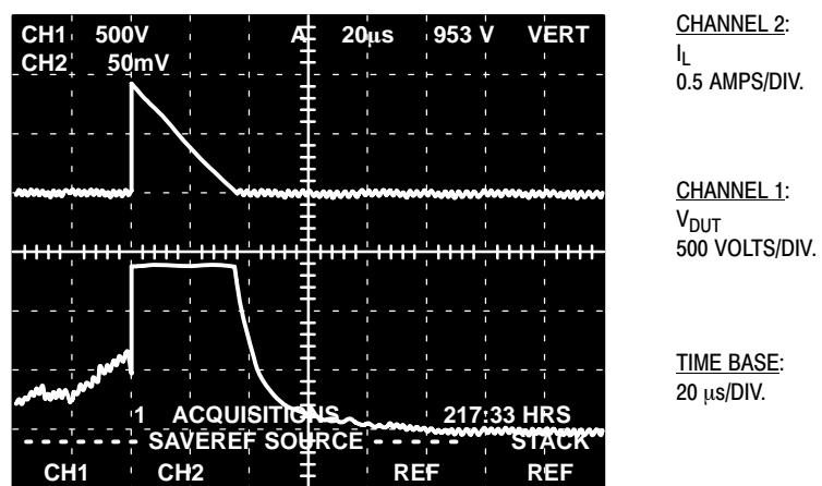
**Figure 8. Current–Voltage Waveforms**
