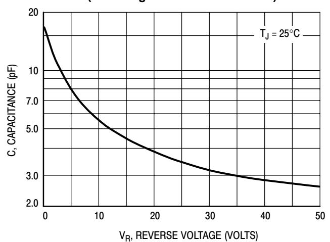
Figure 5. Typical Capacitance
