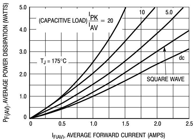
Figure 4. Power Dissipation
