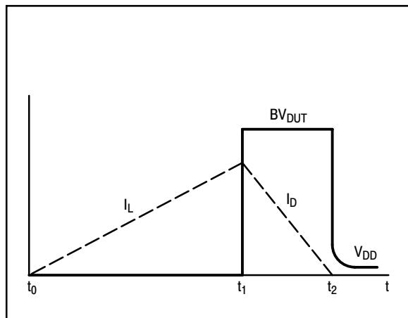
**Figure 7. Current–Voltage Waveforms**
