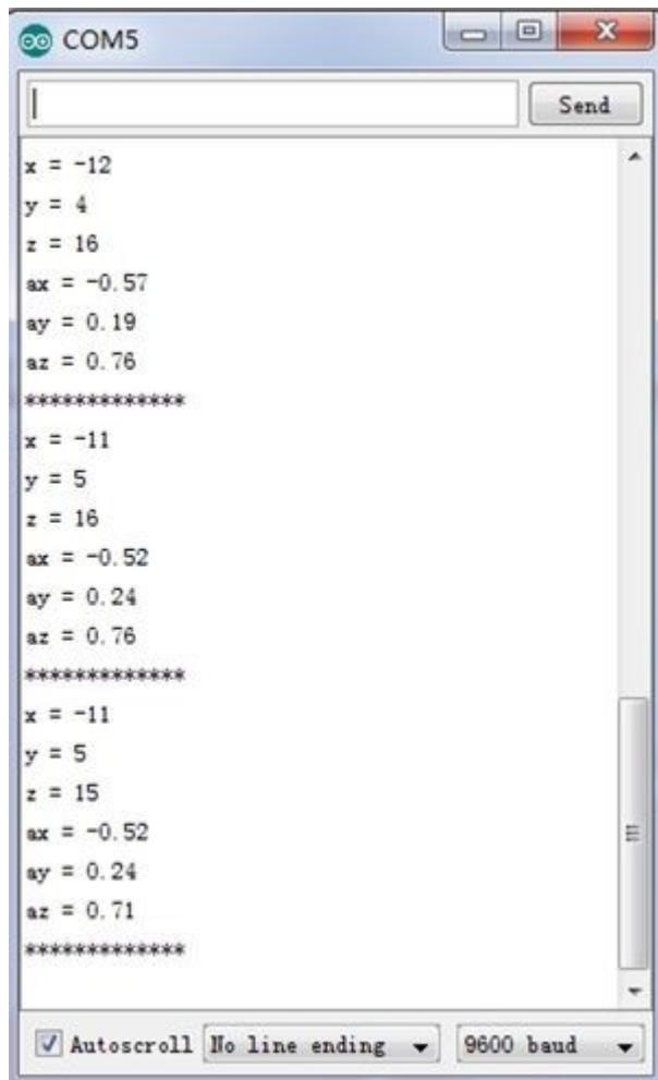
The outputs of this sensor consist of two parts: raw data and 3-axis acceleration info converted into the unit of gravity, "g".
