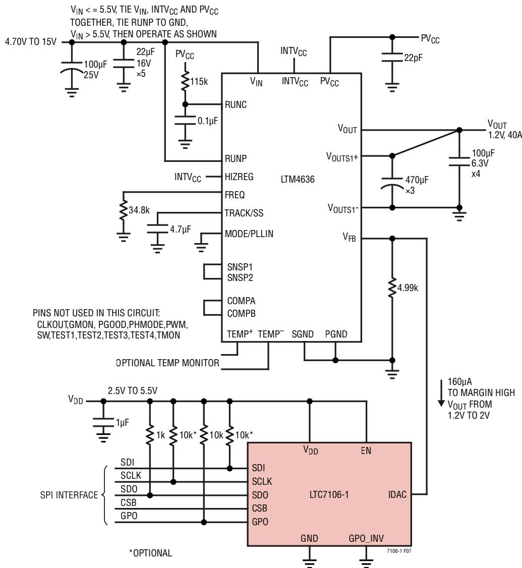
Figure 7. Using the LTC7106-1 to Margin High µModule LTM4636 Providing 1.2V to 2.0V at 40A
