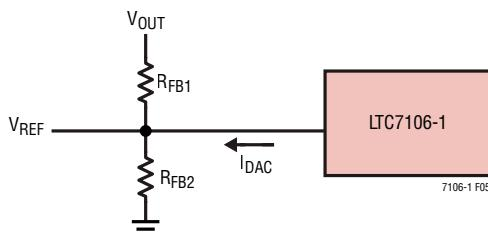
Figure 5. Setting the Output Voltage Using the LTC7106-1
