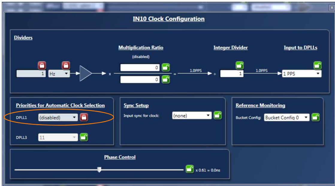
Figure 8. IN10 is disabled as an input clock to DPLL (orange oval)
