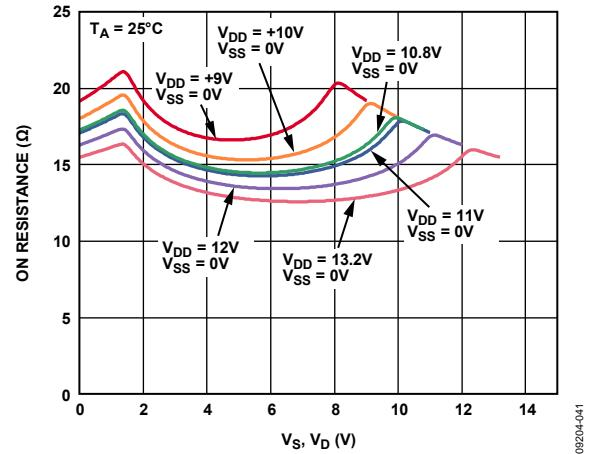
Figure 7. On Resistance vs.  $V_S$ ,  $V_D$  (Single Supply)
