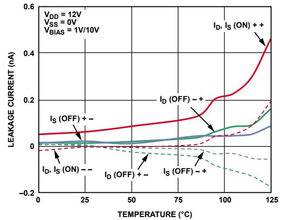
Figure 15. Leakage Currents vs. Temperature, 12 V Single Supply
