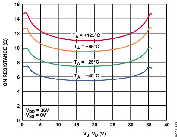
Figure 12. On Resistance vs.  $V_S$  ( $V_D$ ) for Different Temperatures, 36 V Single Supply
