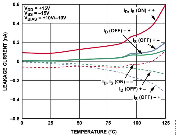
Figure 13. Leakage Currents vs. Temperature, ±15 V Dual Supply
