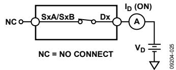
Figure 24. On Leakage
