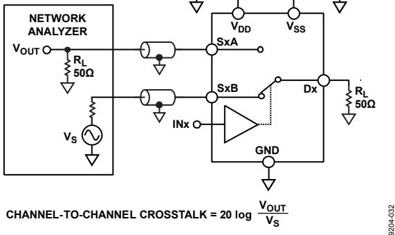
Figure 26. Channel-to-Channel Crosstalk
