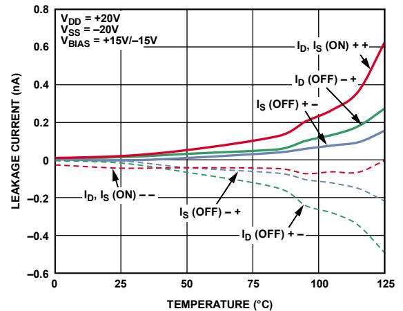
Figure 14. Leakage Currents vs. Temperature, ±20 V Single Supply
