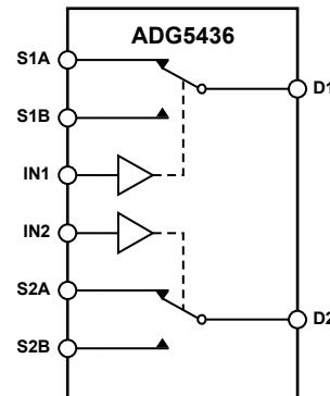
SWITCHES SHOWN FOR A LOGIC 1 INPUT. 09204-001
