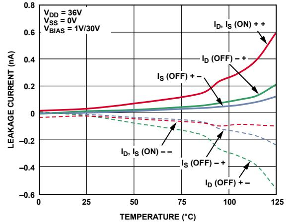
Figure 16. Leakage Currents vs. Temperature, 36 V Single Supply
