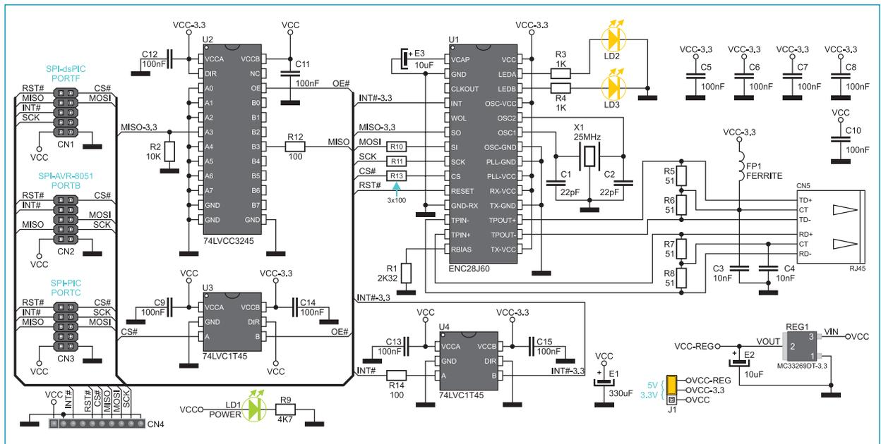
Figure 3: Serial Ethernet additional board connection schematic
