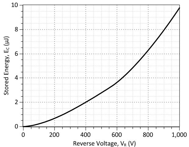
**Figure 4: Typical Switching Energy vs Reverse Voltage Characteristics**
