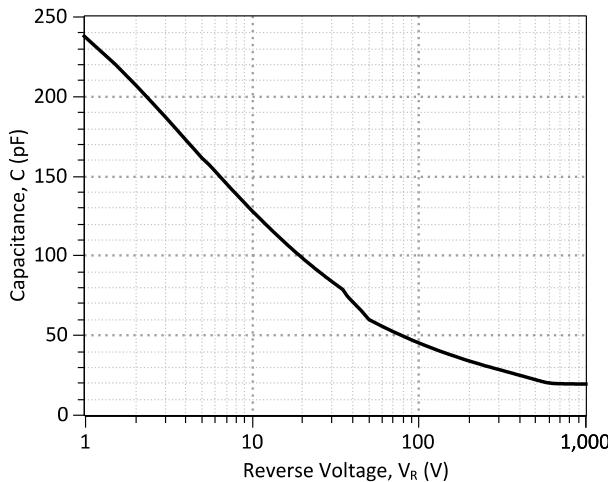
**Figure 3: Typical Junction Capacitance vs Reverse Voltage Characteristics**
