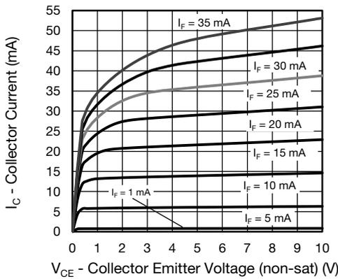
Fig. 6 - Collector Current vs. Collector Emitter Voltage (NS)
