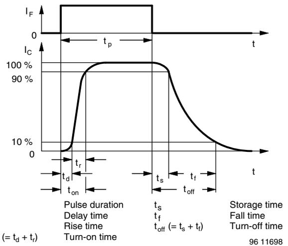
Fig. 4 - Switching Times
