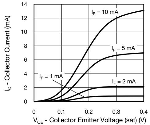
Fig. 8 - Collector Current vs. Collector Emitter Voltage (sat)
