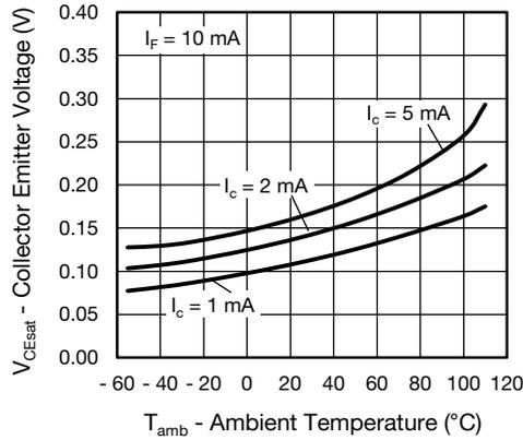
Fig. 11 - Collector Emitter Voltage vs. Ambient Temperature (saturated)
