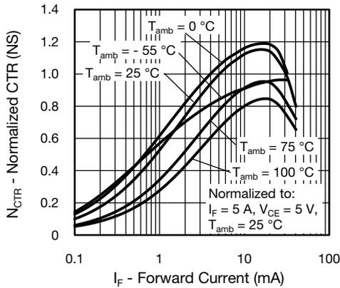
Fig. 12 - Normalized CTR (NS) vs. Forward Current
