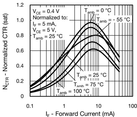
Fig. 13 - Normalized CTR (sat) vs. Forward Current
