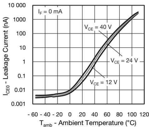
Fig. 7 - Leakage Current vs. Ambient Temperature
