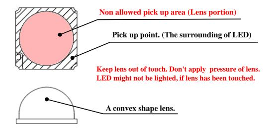
Please adjust the load, the pick up point, the nozzle diameter, etc. before mounting because the over load can cause the breakage of the surrounding of LED.
