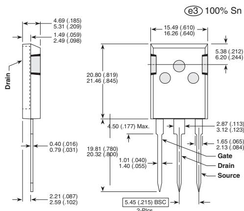
These dimensions are equal to the TO-247 without the mounting hole.
