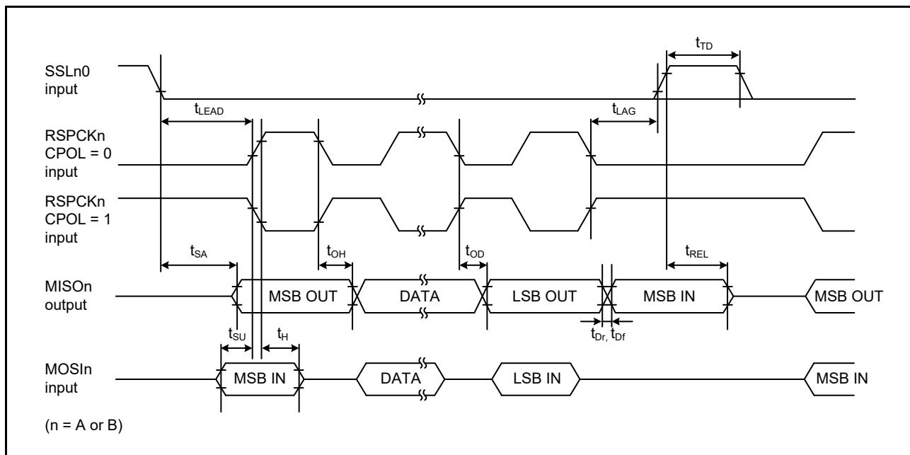
Figure 2.66 SPI timing (slave, CPHA = 0)
