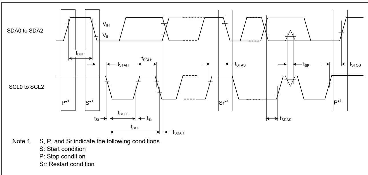
Figure 2.70 I<sup>2</sup>C bus interface input/output timing
