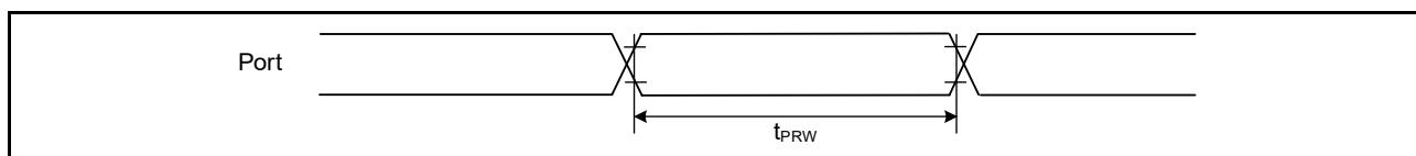
**Figure 2.47 I/O ports input timing**
