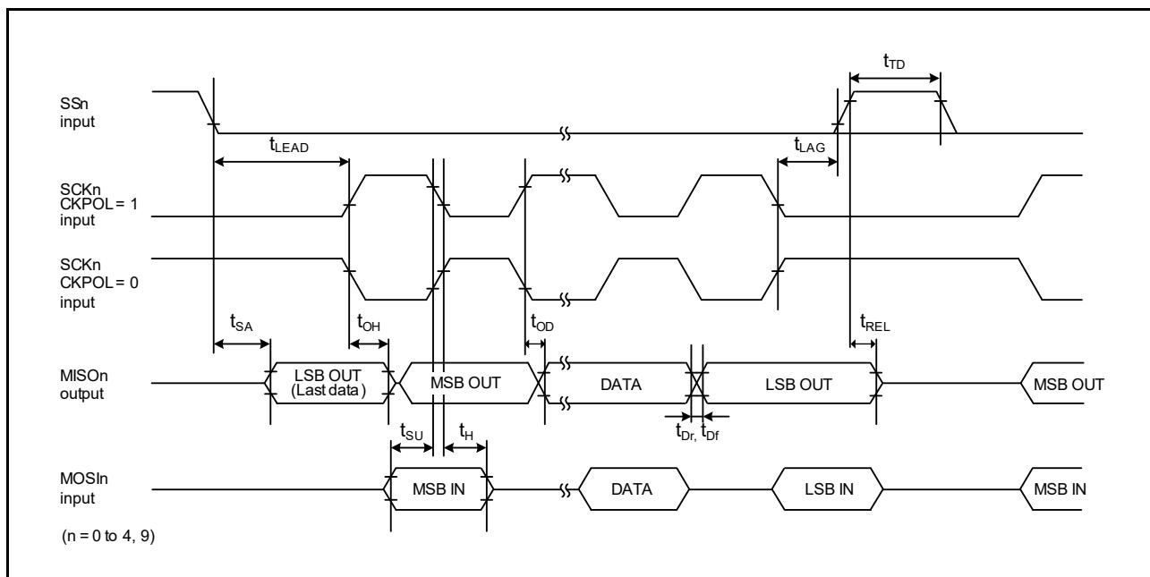
Figure 2.59 SCI simple SPI mode timing (slave, CKPH = 0)
