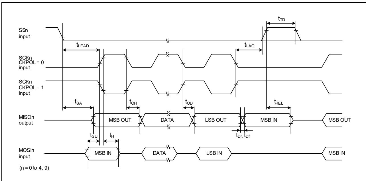
Figure 2.58 SCI simple SPI mode timing (slave, CKPH = 1)
