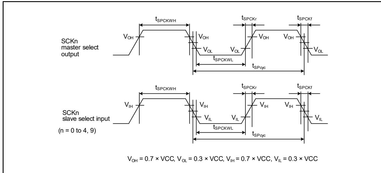
**Figure 2.55 SCI simple SPI mode clock timing**
