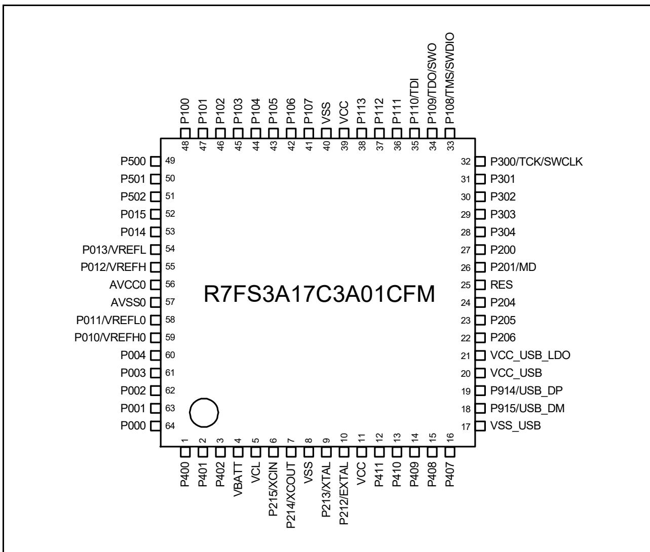
Figure 1.8 Pin assignment for 64-pin LQFP (top view)
