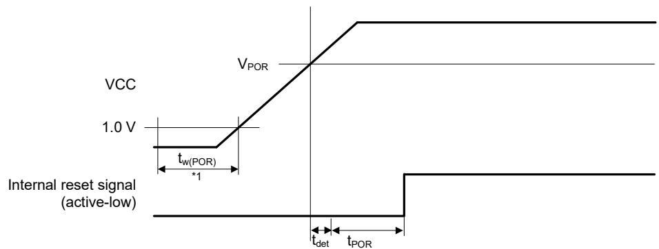
**Figure 2.86** Power-on reset timing
