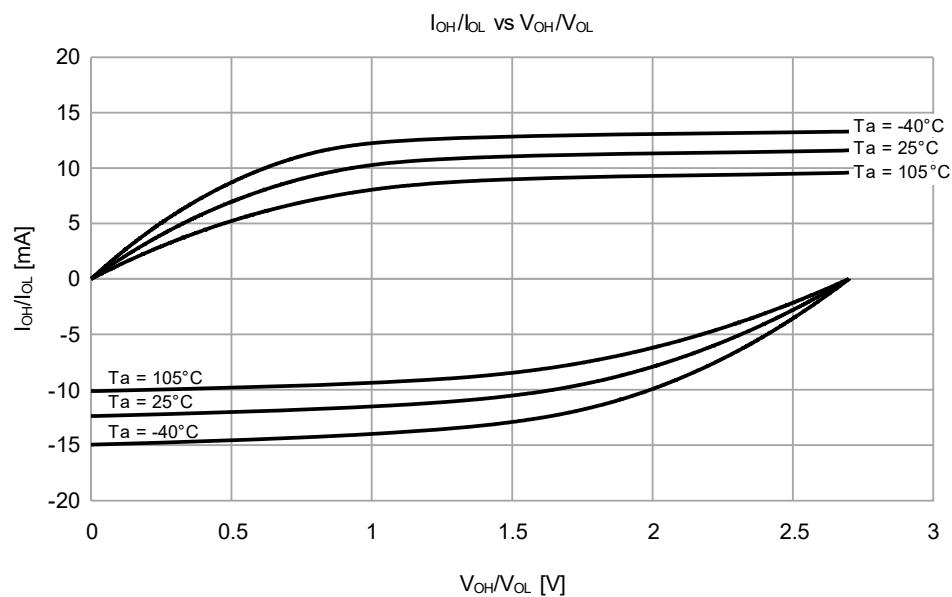
**Figure 2.4**  $V_{OH}/V_{OL}$  and  $I_{OH}/I_{OL}$  temperature characteristics at  $VCC = 2.7$  V when low drive output is selected (reference data)
