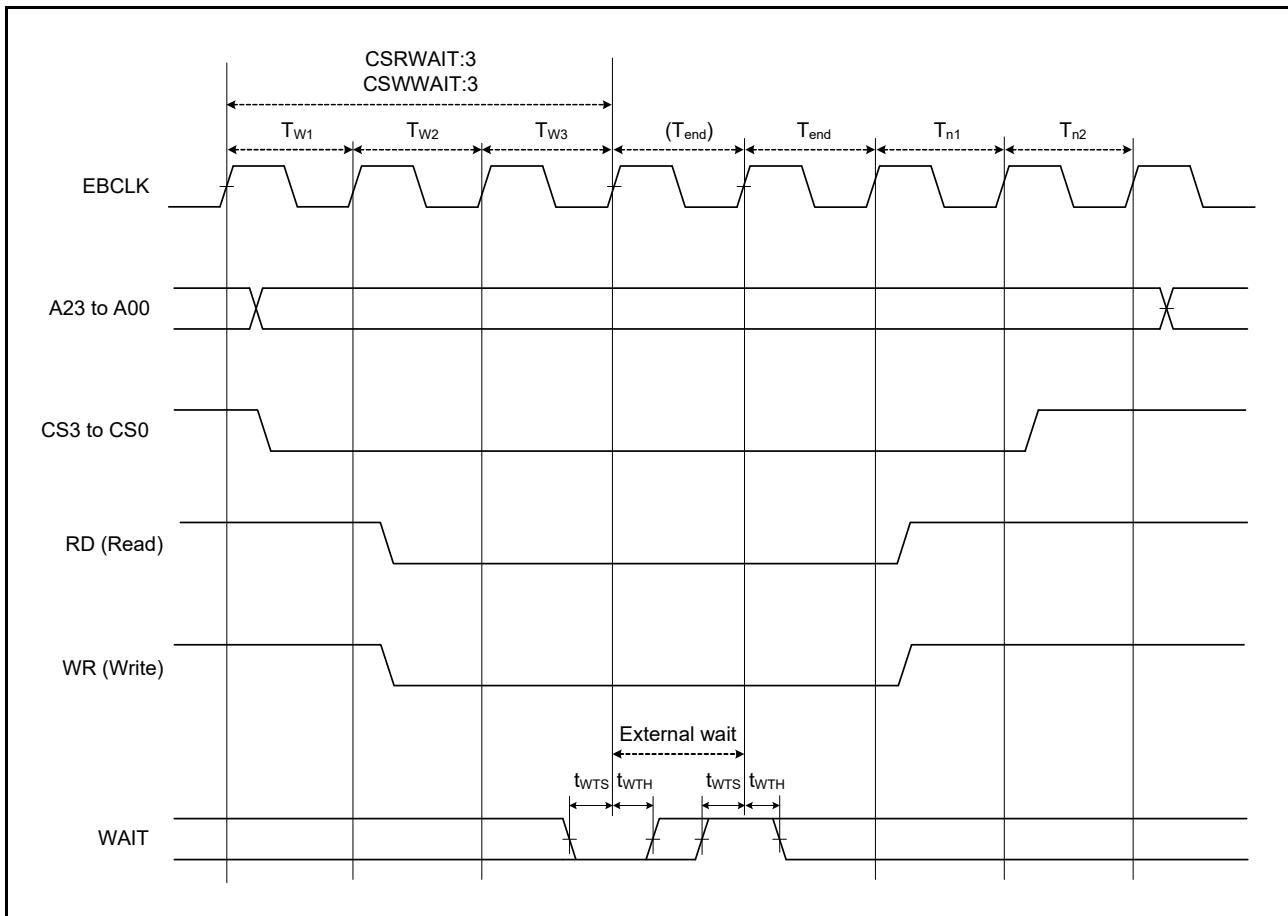
**Figure 2.46 External bus timing/external wait control**
