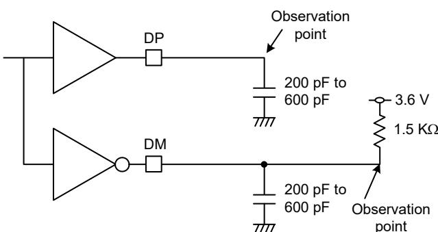
Figure 2.79 Test circuit for Low-Speed (LS) connection
