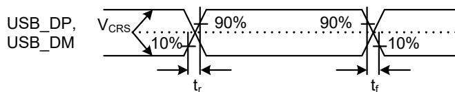
**Figure 2.77** USB\_DP and USB\_DM output timing
