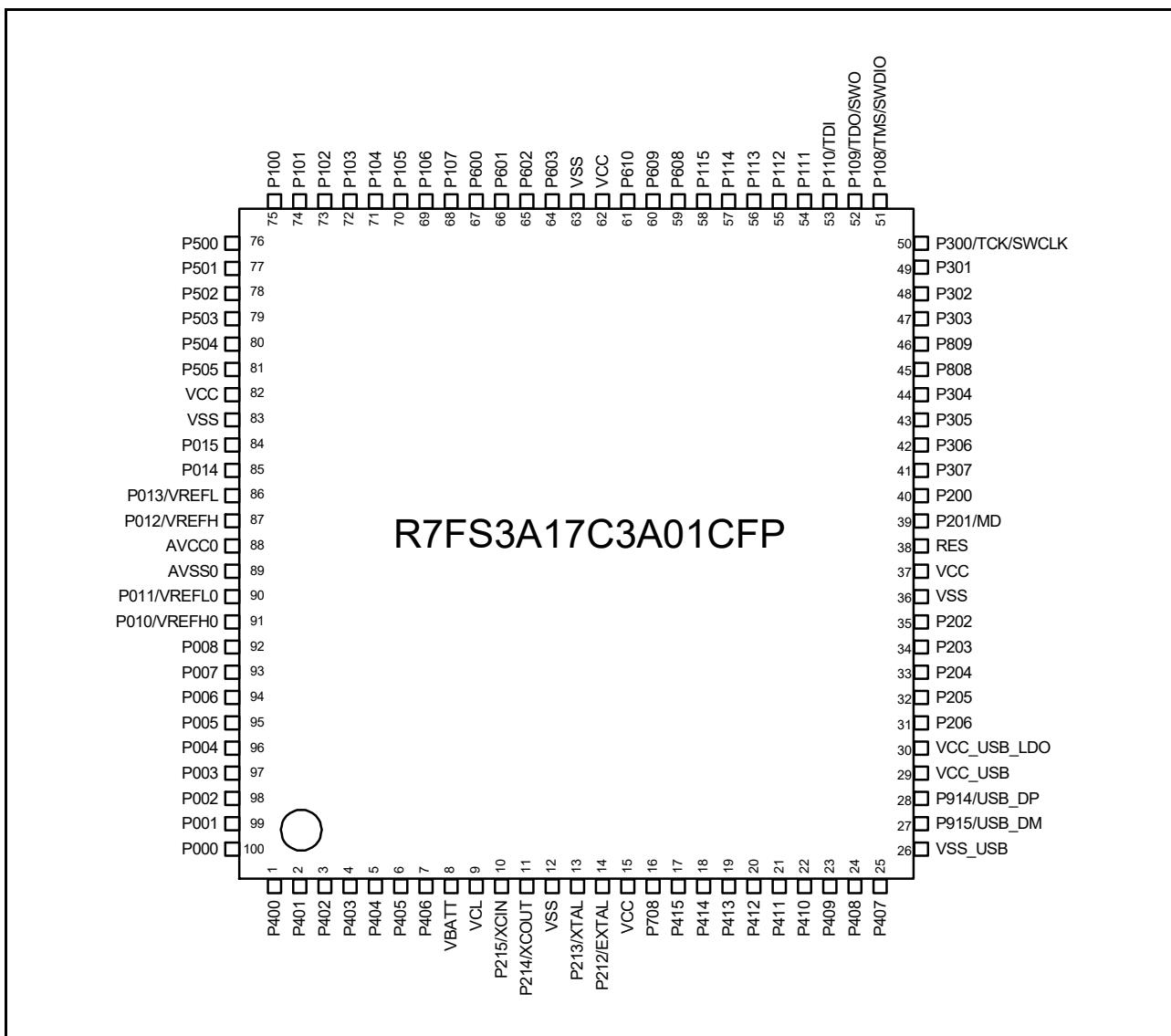
Figure 1.6 Pin assignment for 100-pin LQFP (top view)
