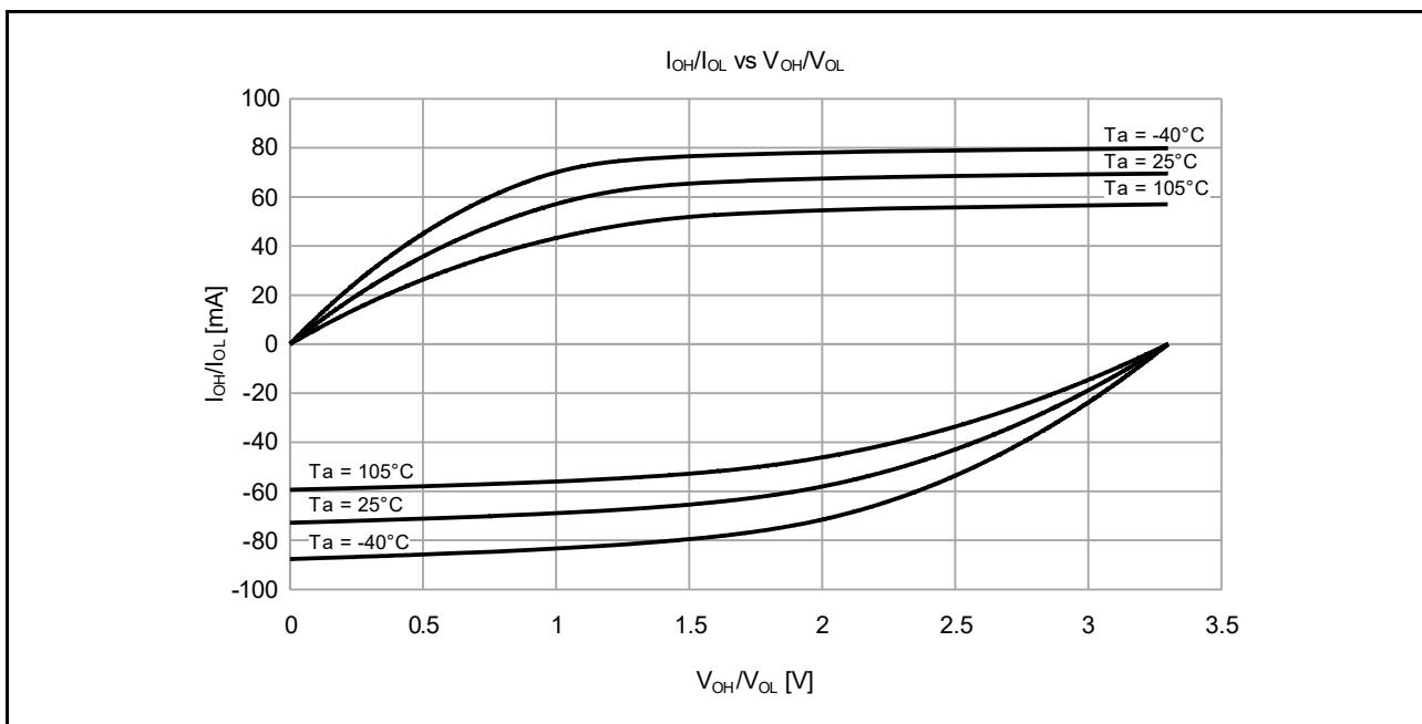
**Figure 2.14** V<sub>OH</sub>/V<sub>OL</sub> and I<sub>OH</sub>/I<sub>OL</sub> temperature characteristics at VCC = 3.3 V when middle drive output is selected (reference data)
