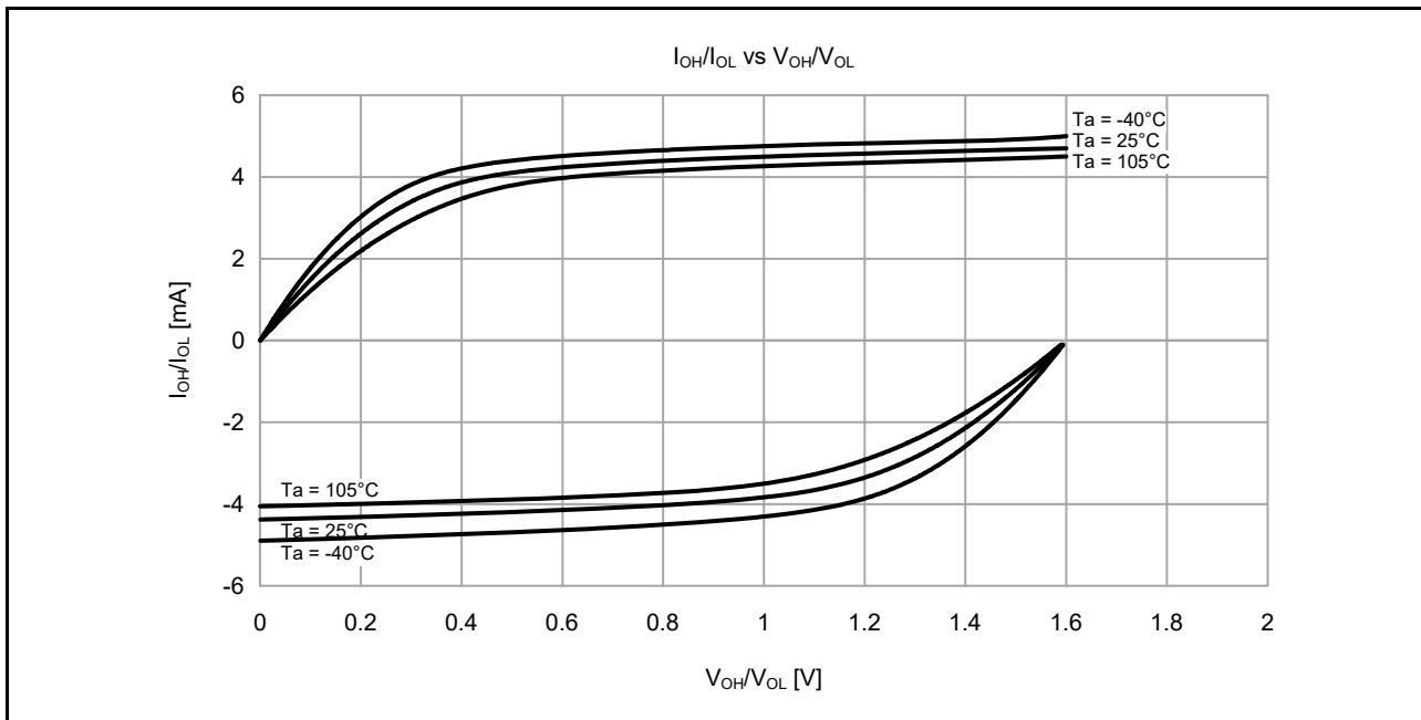
**Figure 2.8** V<sub>OH</sub>/V<sub>OL</sub> and I<sub>OH</sub>/I<sub>OL</sub> temperature characteristics at VCC = 1.6 V when middle drive output is selected (reference data)
