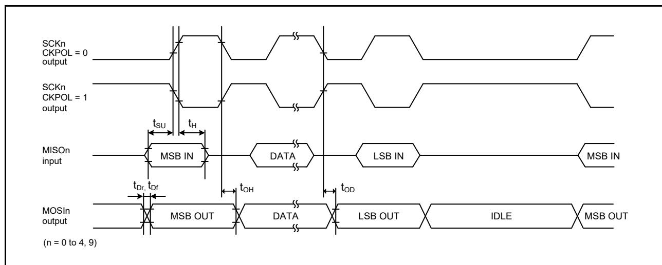
**Figure 2.56 SCI simple SPI mode timing (master, CKPH = 1)**
