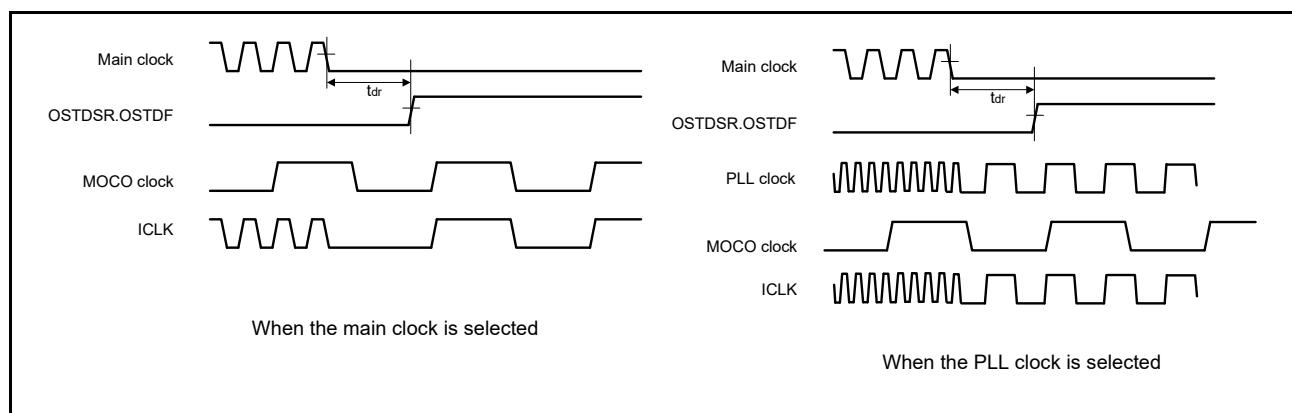
**Figure 2.84 Oscillation stop detection timing**
