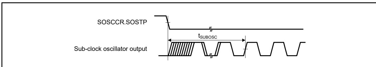
Figure 2.32 Sub-clock oscillation start timing
