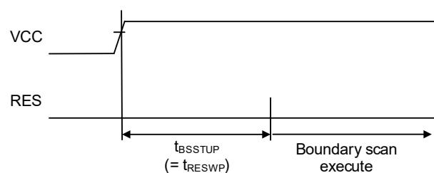
Figure 2.96 Boundary scan circuit start up timing
