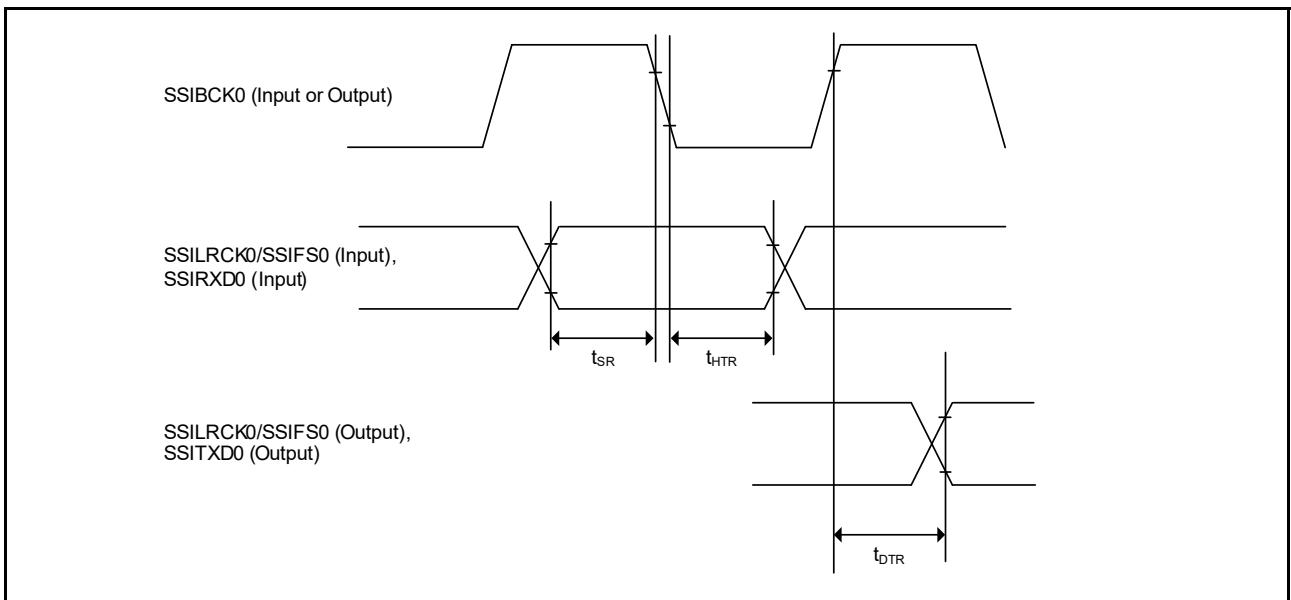
Figure 2.73 SSIE data transmit/receive timing (SSICR.BCKP = 1)
