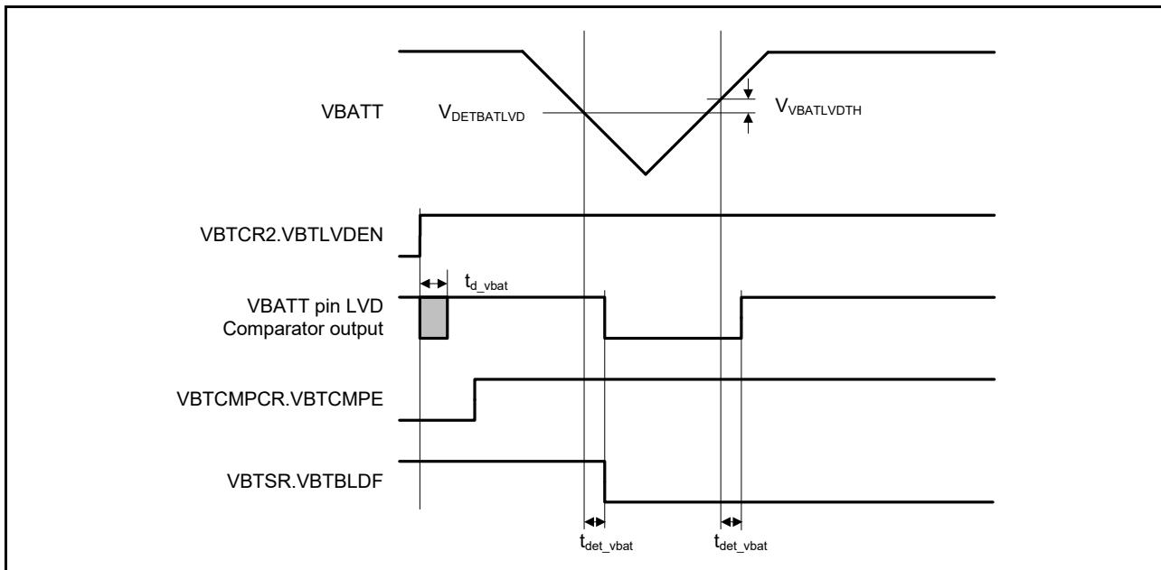
Figure 2.92 VBATT pin voltage detection circuit timing
