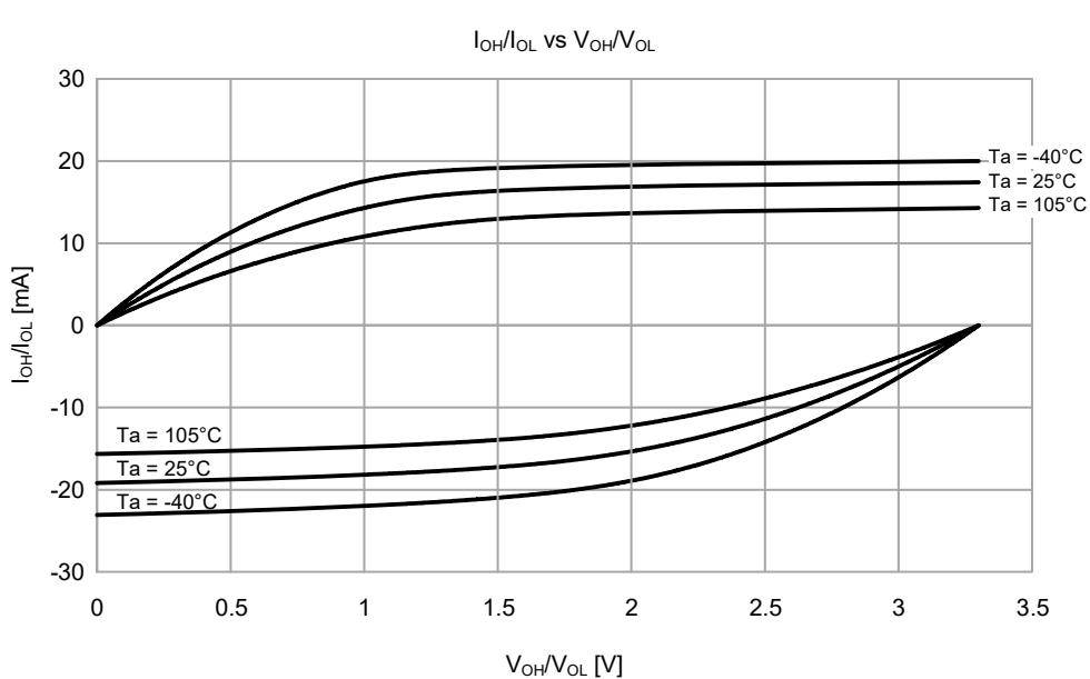
**Figure 2.5**  $V_{OH}/V_{OL}$  and  $I_{OH}/I_{OL}$  temperature characteristics at  $VCC = 3.3$  V when low drive output is selected (reference data)
