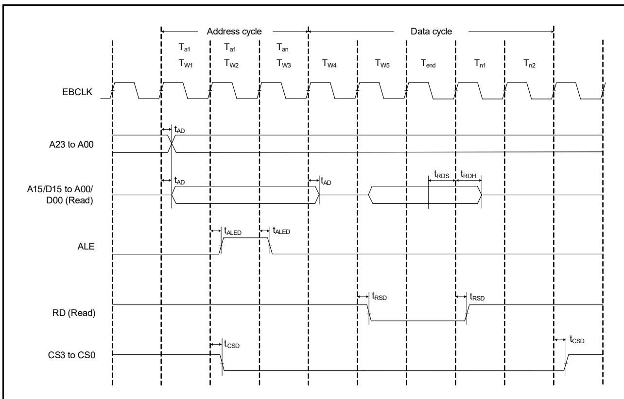
Figure 2.40 Address/data multiplexed bus read access timing
