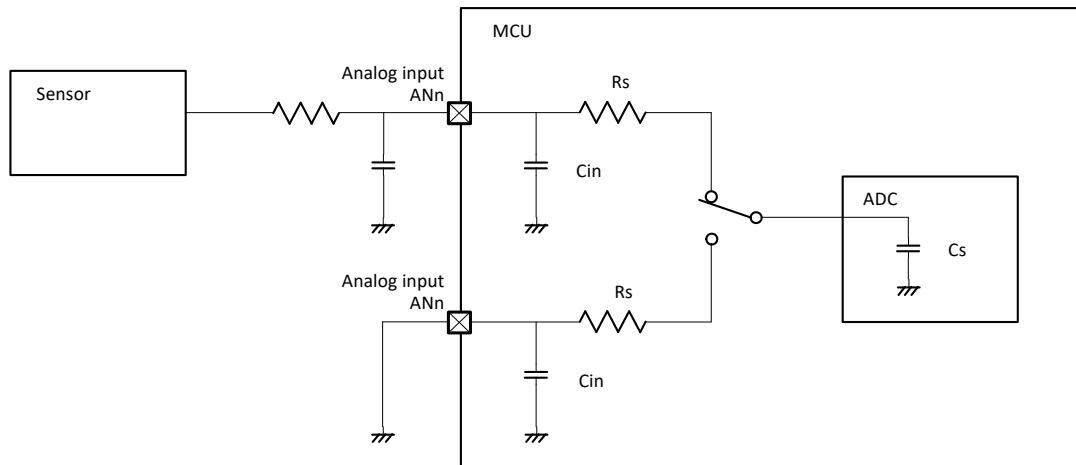
**Figure 2.81** Equivalent circuit for analog input**Table 2.55** 14-bit A/D converter channel classification
