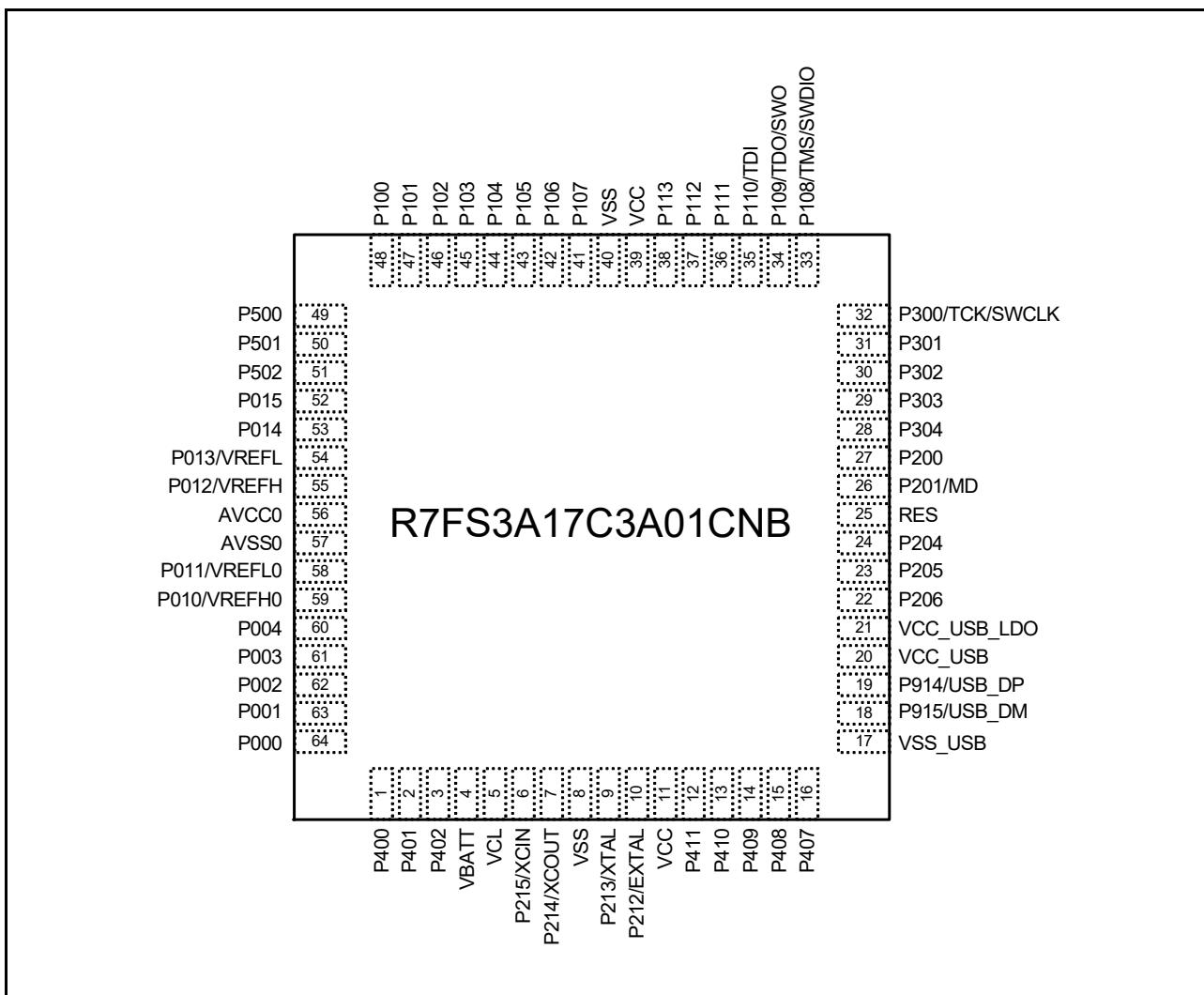
Figure 1.9 Pin assignment for 64-pin QFN (top view)
