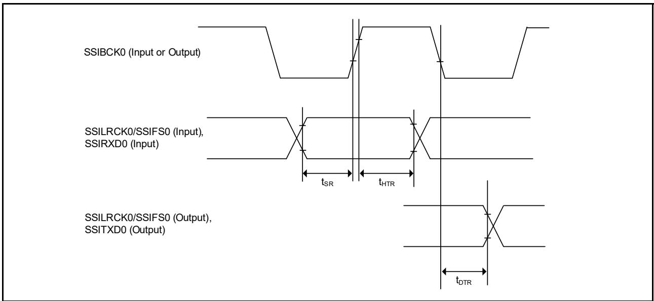
Figure 2.72 SSIE data transmit/receive timing (SSICR.BCKP = 0)
