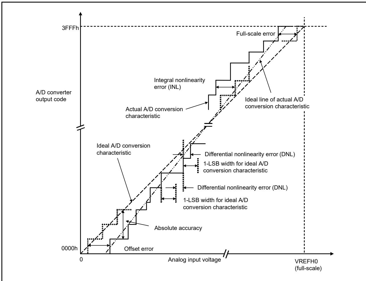
**Figure 2.82 Illustration of 14-bit A/D converter characteristic terms**
