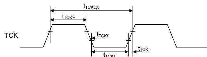
Figure 2.94 Boundary scan TCK timing
