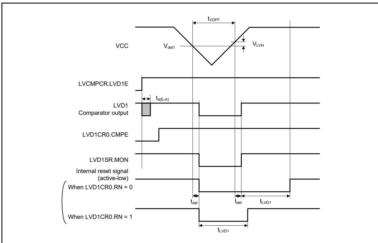
Figure 2.88 Voltage detection circuit timing ( $V_{det1}$ )
