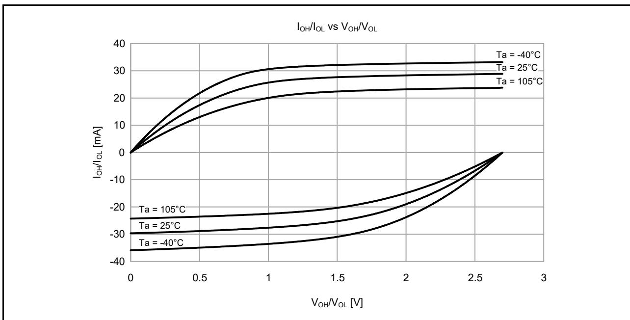
**Figure 2.9** V<sub>OH</sub>/V<sub>OL</sub> and I<sub>OH</sub>/I<sub>OL</sub> temperature characteristics at VCC = 2.7 V when middle drive output is selected (reference data)
