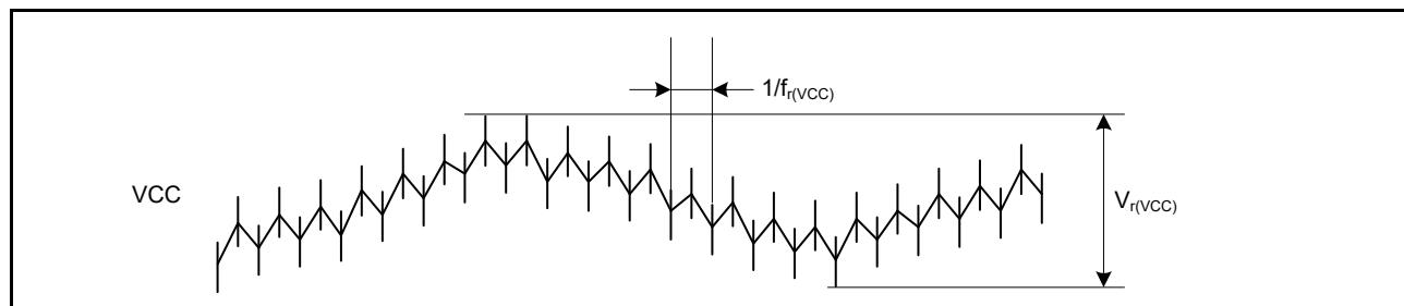
**Figure 2.25 Ripple waveform**
