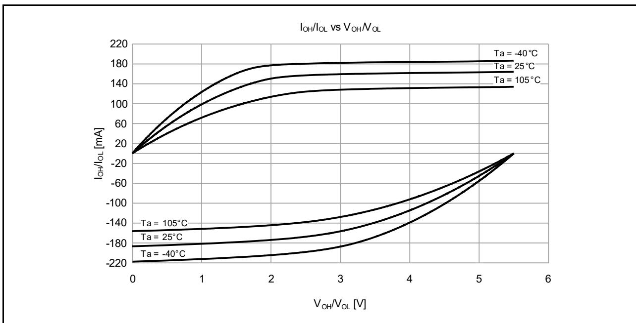
**Figure 2.15** V<sub>OH</sub>/V<sub>OL</sub> and I<sub>OH</sub>/I<sub>OL</sub> temperature characteristics at VCC = 5.5 V when middle drive output is selected (reference data)
