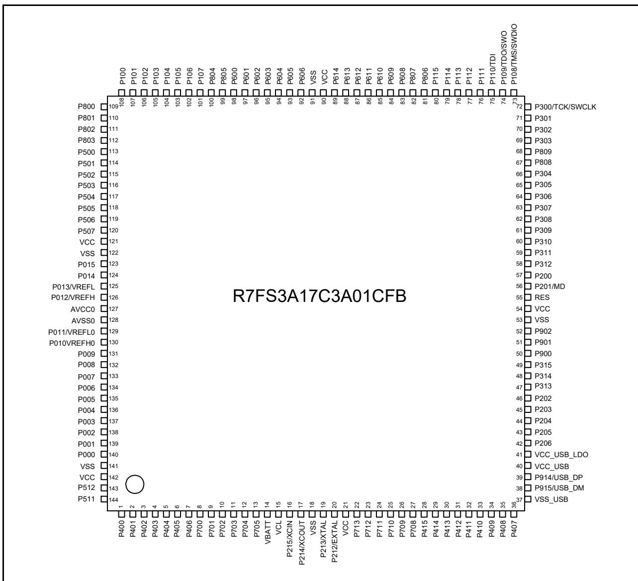
**Figure 1.4 Pin assignment for 144-pin LQFP (top view)**
