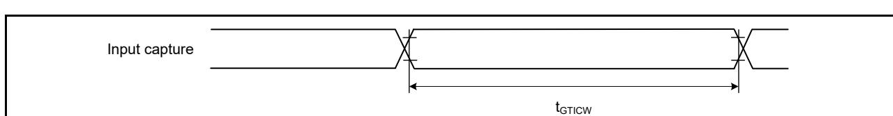
**Figure 2.49 GPT input capture timing**
