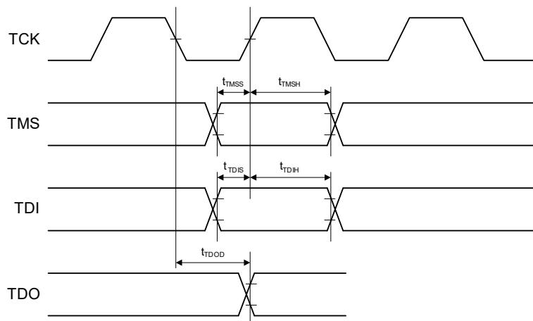
Figure 2.95 Boundary scan input/output timing
