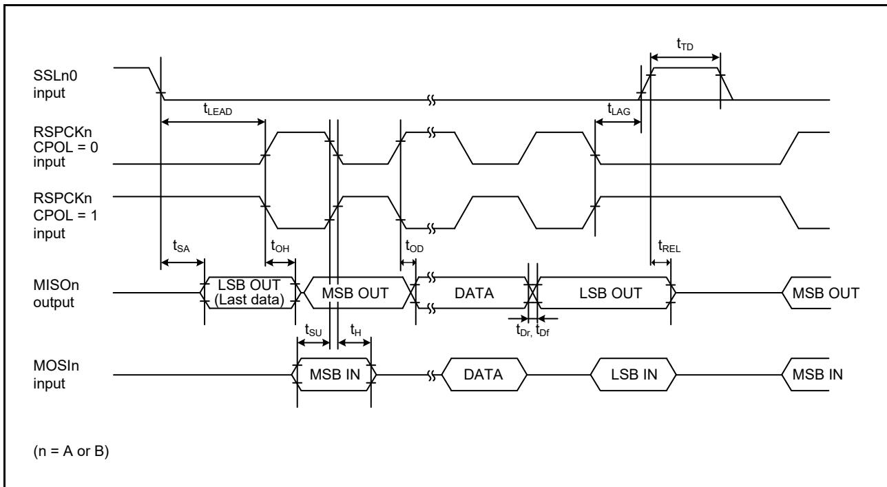
Figure 2.67 SPI timing (slave, CPHA = 1)
