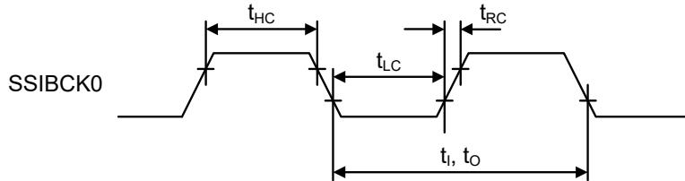
**Figure 2.71 SSIE clock input/output timing**
