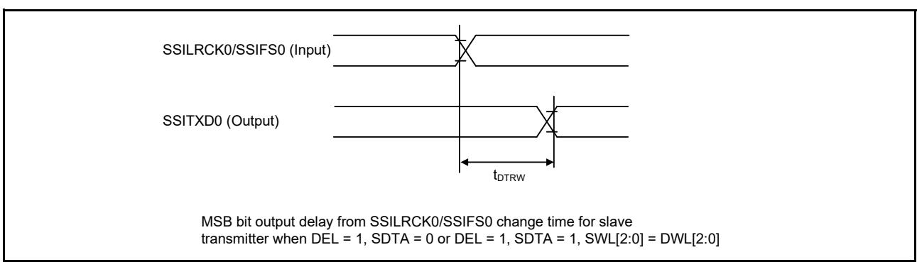
Figure 2.74 SSIE data output delay from SSILRCK0/SSIIFS0 change time
