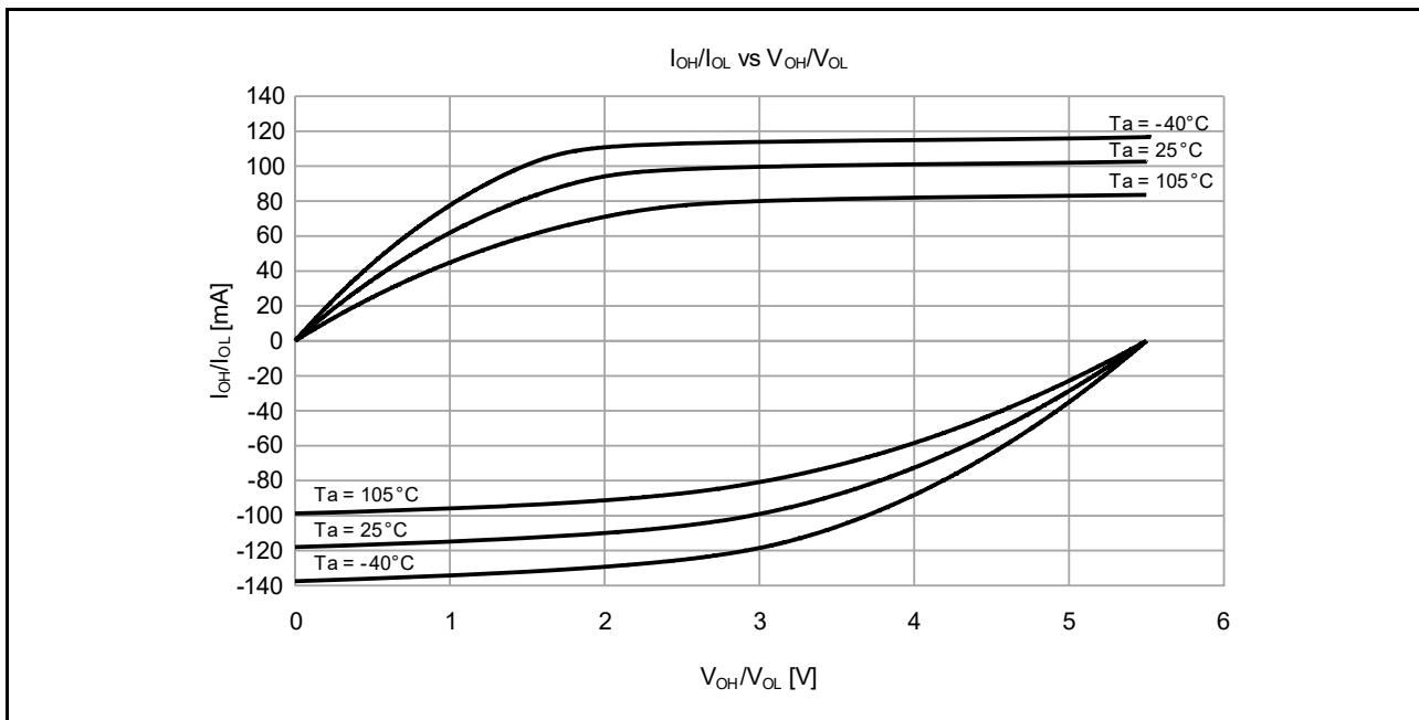
**Figure 2.11** V<sub>OH</sub>/V<sub>OL</sub> and I<sub>OH</sub>/I<sub>OL</sub> temperature characteristics at VCC = 5.5 V when middle drive output is selected (reference data)
