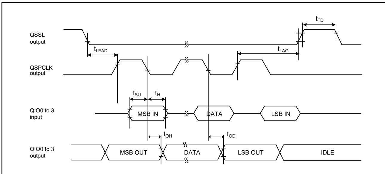
**Figure 2.69** Transfer/receive timing
