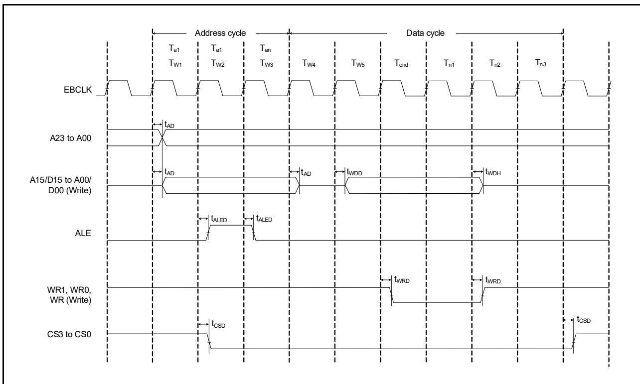
Figure 2.41 Address/data multiplexed bus write access timing
