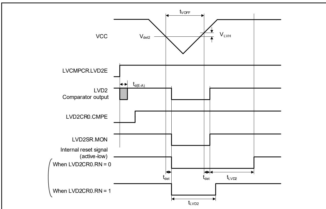
Figure 2.89 Voltage detection circuit timing ( $V_{det2}$ )
