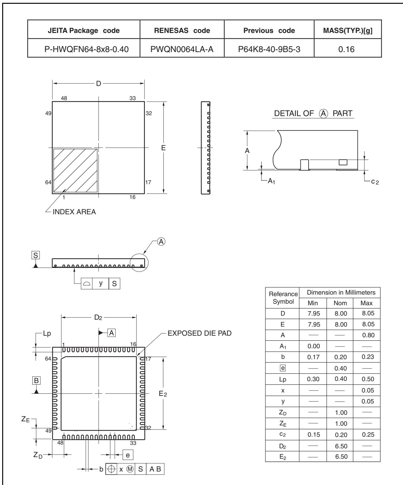
Figure 1.7 QFN 64-pin
