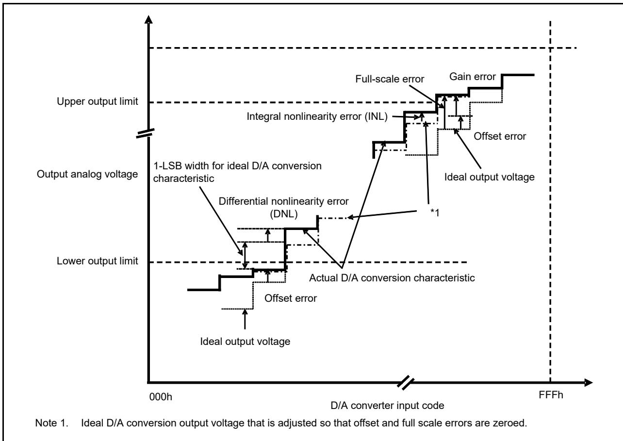
**Figure 2.83 Illustration of D/A converter characteristic terms**
