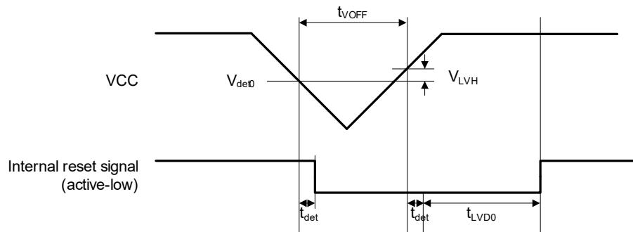
**Figure 2.87** Voltage detection circuit timing ( $V_{det0}$ )
