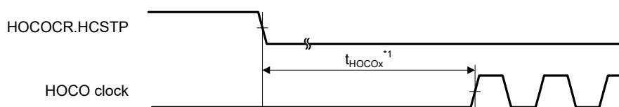
Figure 2.29 HOCO clock oscillation start timing (started by setting HOCOCR.HCSTP bit)
