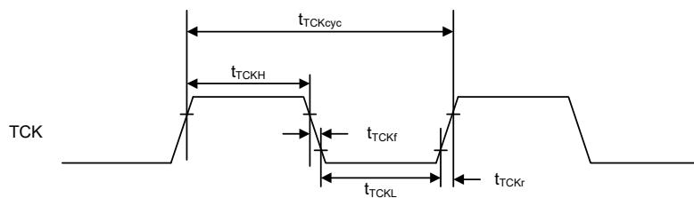
**Figure 2.97 JTAG TCK timing**
