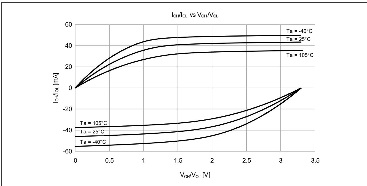
**Figure 2.10** V<sub>OH</sub>/V<sub>OL</sub> and I<sub>OH</sub>/I<sub>OL</sub> temperature characteristics at VCC = 3.3 V when middle drive output is selected (reference data)
