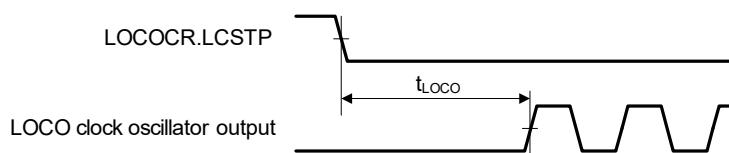
Figure 2.28 LOCO clock oscillation start timing
