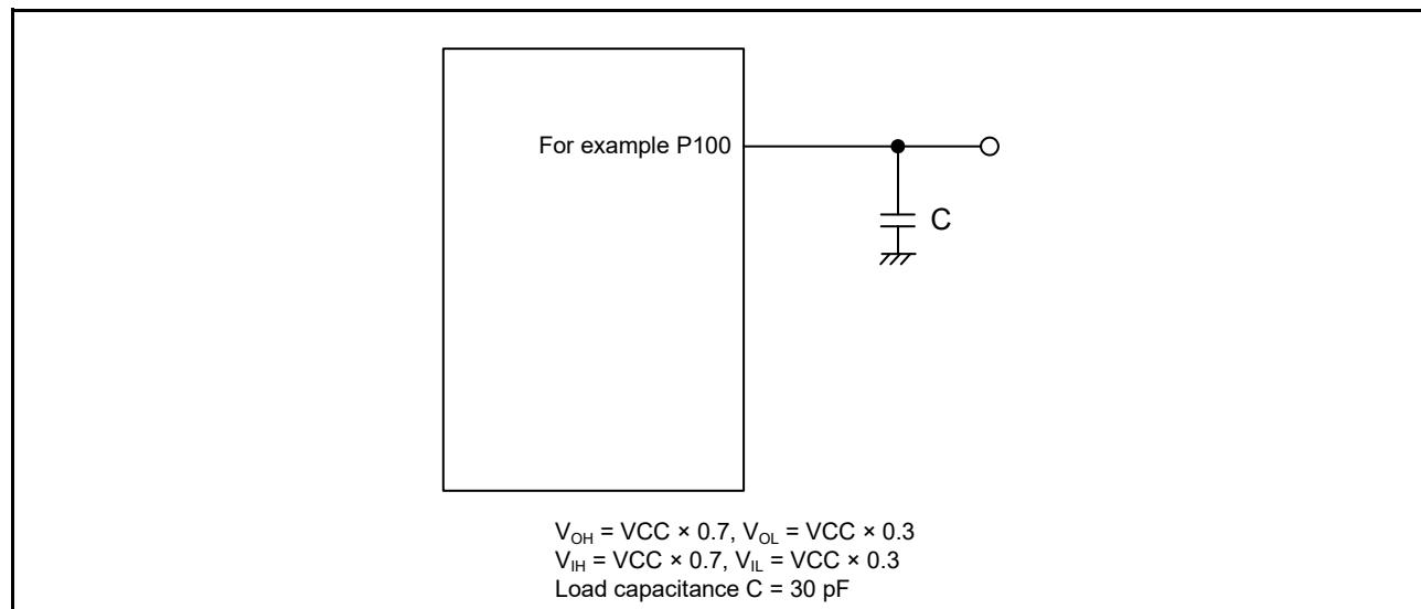
**Figure 2.1 Input or output timing measurement conditions**
