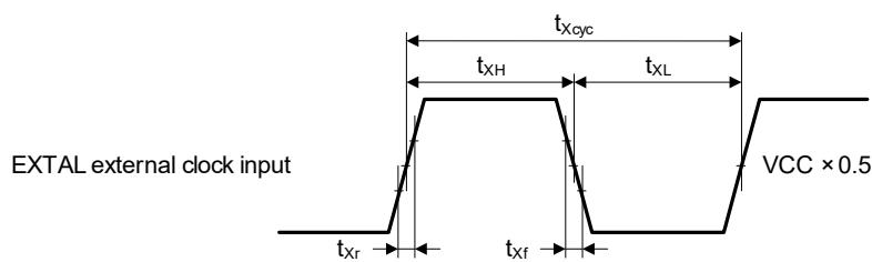
Figure 2.27 EXTAL external clock input timing
