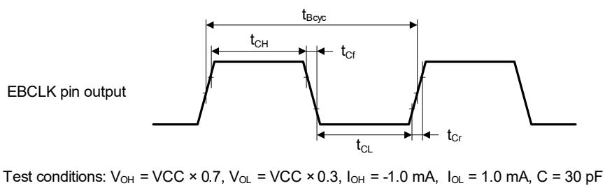
Figure 2.26 EBCLK pin output timing
