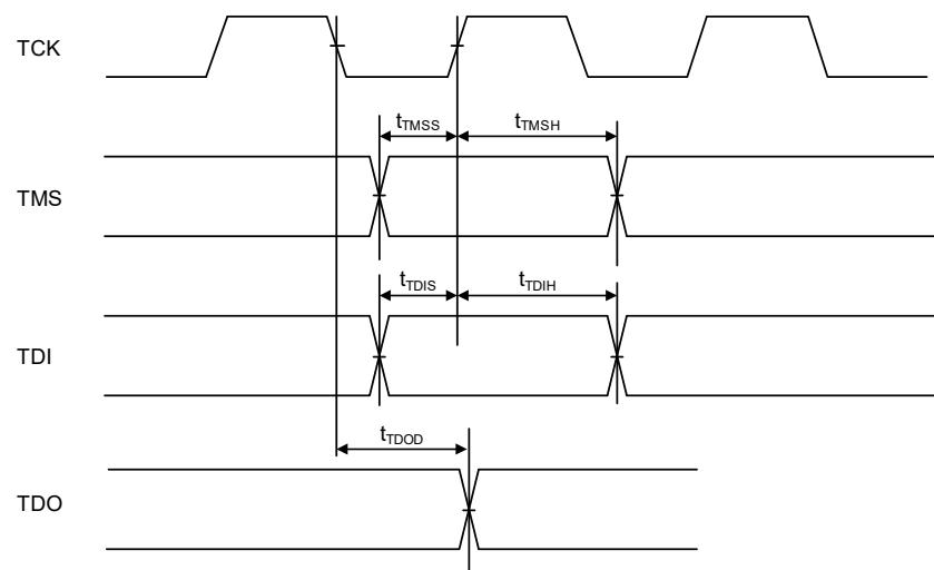
**Figure 2.98 JTAG input/output timing**
