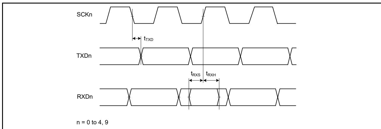
Figure 2.54 SCI input/output timing in clock synchronous mode
