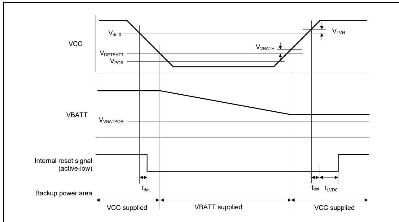
**Figure 2.90 Power supply switching and LVD0 reset timing**
