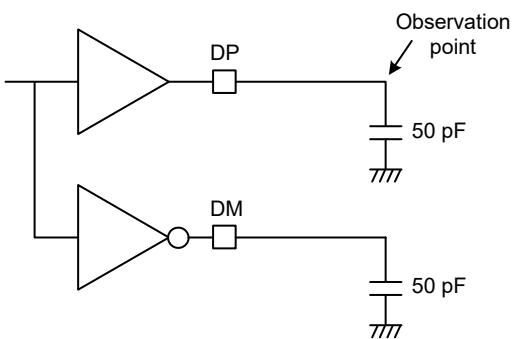
Figure 2.78 Test circuit for Full-Speed (FS) connection
