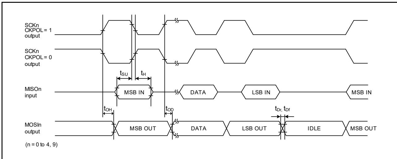
Figure 2.57 SCI simple SPI mode timing (master, CKPH = 0)
