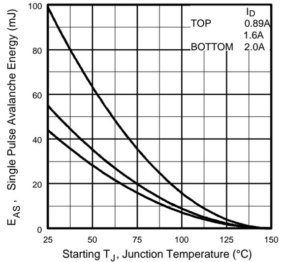
**Fig 8.** Maximum Avalanche Energy Vs. Drain Current
