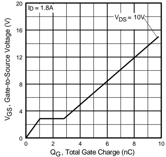
**Fig 10.** Typical Gate Charge Vs. Gate-to-Source Voltage
