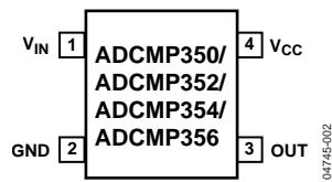
Figure 2. Pin Configuration
