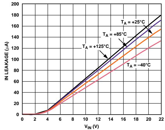
Figure 7. Input Leakage vs. Input Voltage
