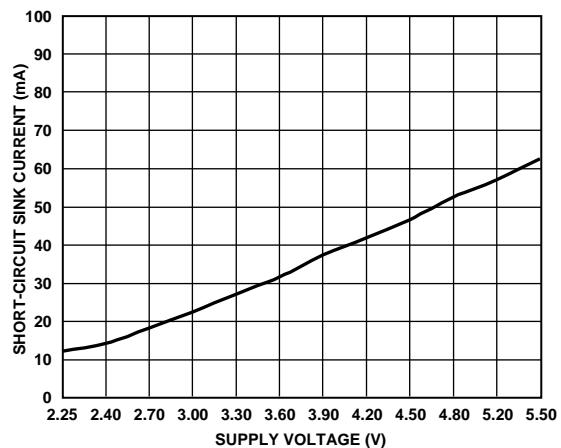
Figure 15. Short-Circuit Sink Current vs. Supply Voltage
