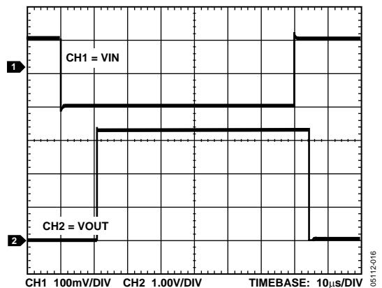
Figure 18. Propagation Delay Timing, 100 mV Overdrive
