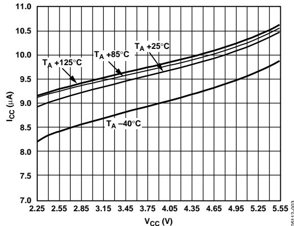
Figure 3.  $I_{CC}$  vs.  $V_{CC}$  over Temperature.
