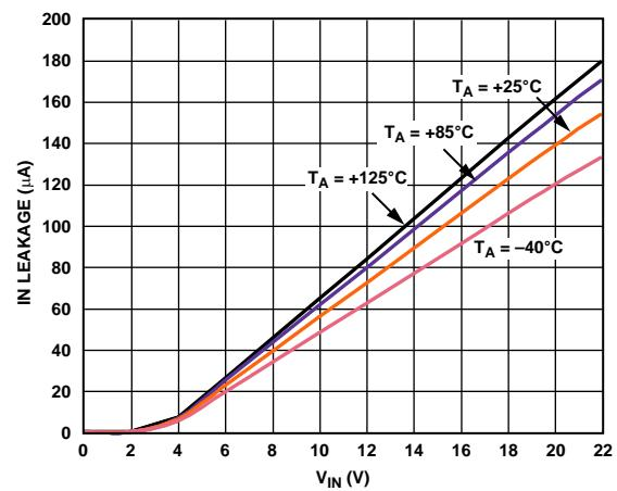
Figure 7. Input Leakage vs. Input Voltage
