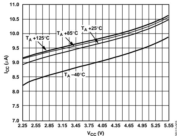
Figure 3.  $I_{CC}$  vs.  $V_{CC}$  over Temperature.
