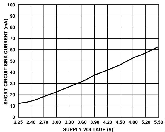
Figure 15. Short-Circuit Sink Current vs. Supply Voltage
