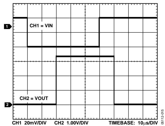
Figure 17. Propagation Delay Timing, 10 mV Overdrive
