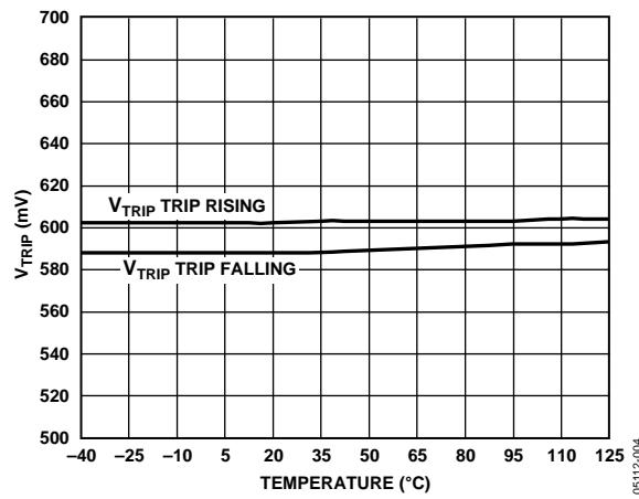
Figure 4.  $V_{IN}$  Trip Threshold vs. Temperature. ( $V_{CC} = 3.3V$ )
