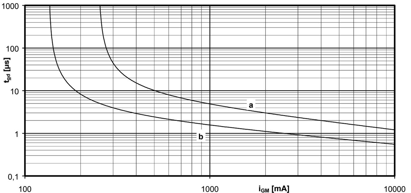
Zündverzug / Gate controlled delay time  $t_{gd} = f(i_{GM})$
