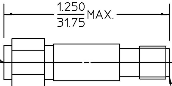
CONNECTOR, RECEPTACLE, FEMALE, SMA TYPE, MATES WITH CONNECTOR, PLUG, MALE PER MIL-C-39012
