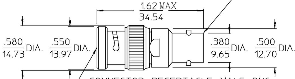
CONNECTOR, RECEPTACLE, MALE, BNC TYPE, MATES WITH CONNECTOR, JACK FEMALE PER MIL-C-39012
