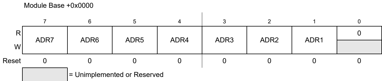
Figure 20-3. IIC Bus Address Register (IBAD)
