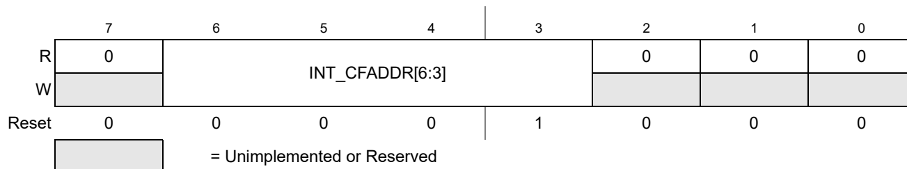
Figure 6-4. Interrupt Configuration Address Register (INT_CFADDR)
