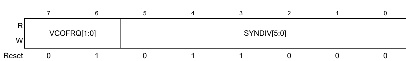
Figure 9-7. S12CPMU_UHV Synthesizer Register (CPMUSYNR)
