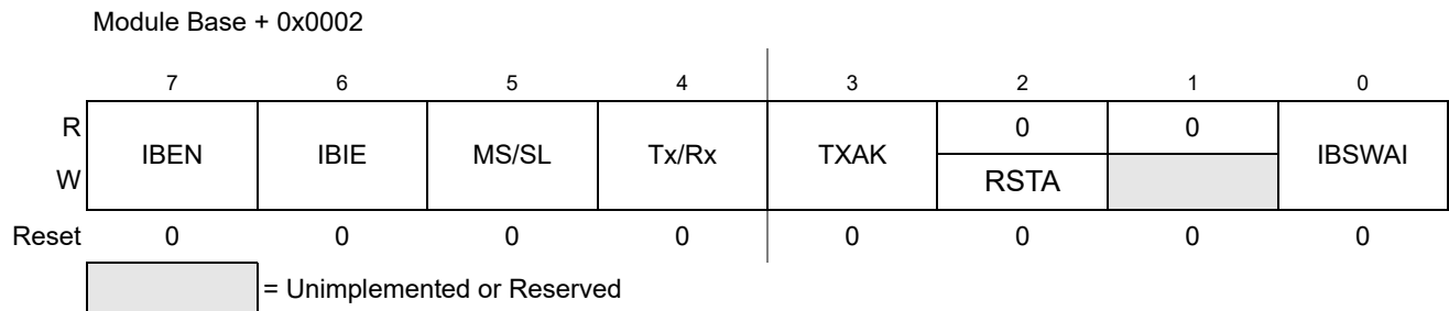
Figure 20-6. IIC Bus Control Register (IBCR)
