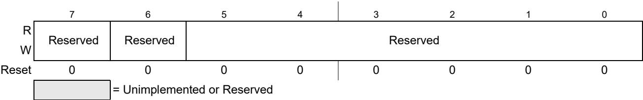
Figure 10-21. ADC Command Register 3 (ADCCMD_3)
