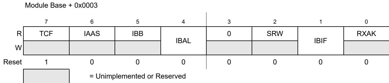
Figure 20-7. IIC Bus Status Register (IBSR)
