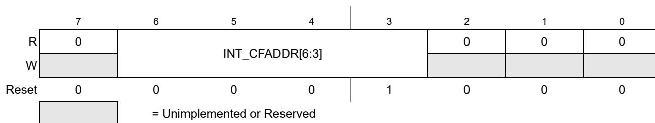
Figure 6-4. Interrupt Configuration Address Register (INT_CFADDR)
