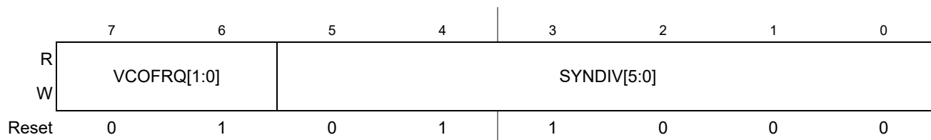
Figure 9-7. S12CPMU_UHV Synthesizer Register (CPMUSYNR)
