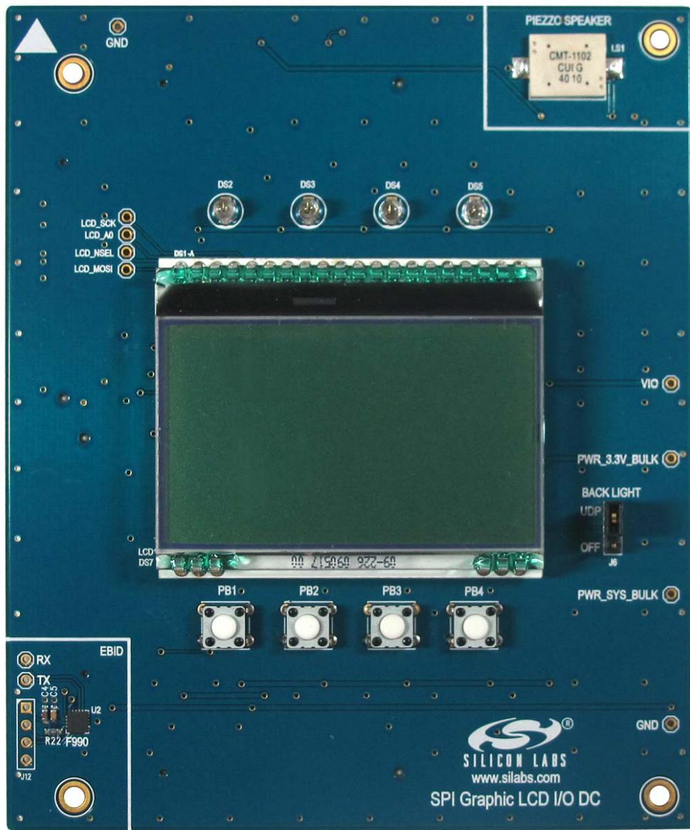
Figure 4. Unified Development Platform Example I/O Card
