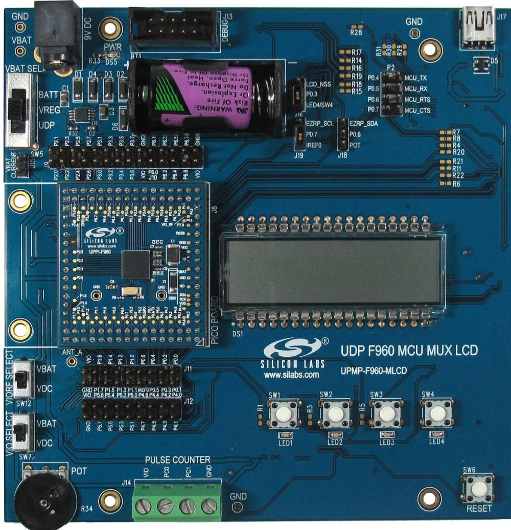
Figure 3. Unified Development Platform Example MCU Card
