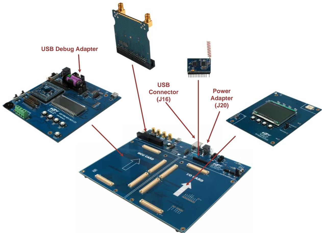
**Figure 7. Hardware Setup using the Unified Development Platform**
