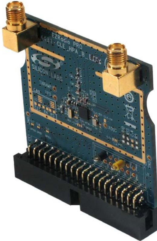
**Figure 5. Unified Development Platform Example Radio Card**
