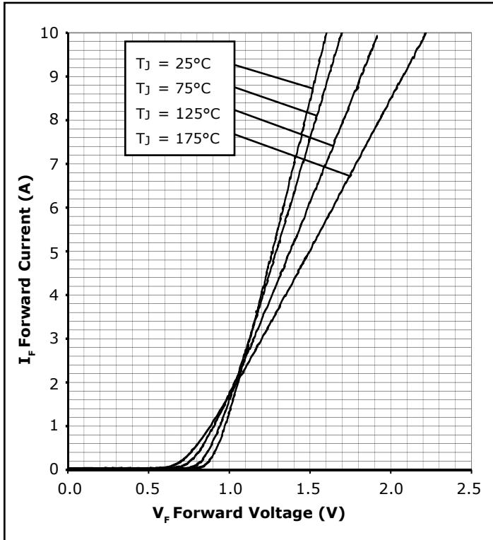
Figure 1. Forward Characteristics
