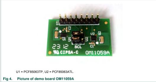
The original version of OM11059A allows to easily demonstrate the operation of the PCF85063x with I<sup>2</sup>C-bus interface. No need to solder the tiny package to a breadboard 100 mil connector for straight forward connections.
