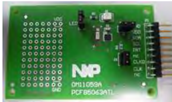
Fig 8. Picture of PCF85063ATL demo board OM11059A
