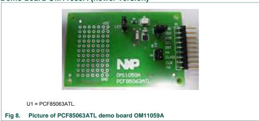
The 2<sup>nd</sup> version of OM11059A allows to easily demonstrate the operation of only the popular PCF85063ATL with I<sup>2</sup>C-bus interface. No need to solder the tiny package to a breadboard 100 mil connector for straight forward connections.
