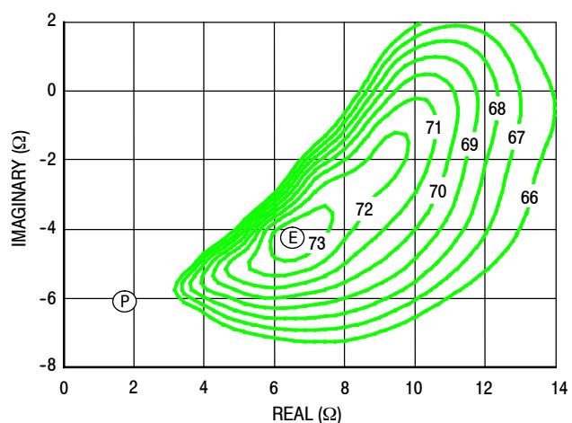
Figure 21. P3dB Load Pull Efficiency Contours (%)
