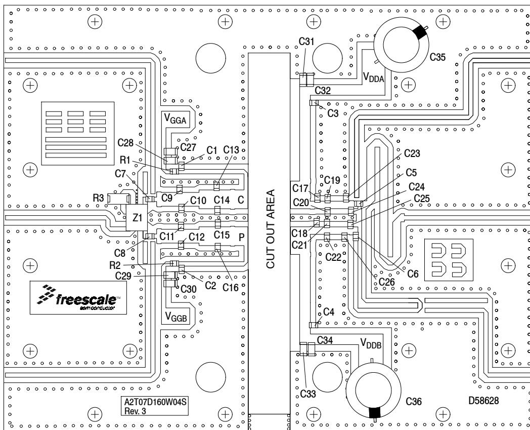
Note: V<sub>DDA</sub> and V<sub>DBB</sub> must be tied together and powered by a single DC power supply.
