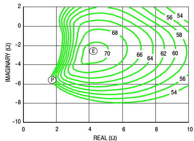
Figure 29. P1dB Load Pull Efficiency Contours (%)
