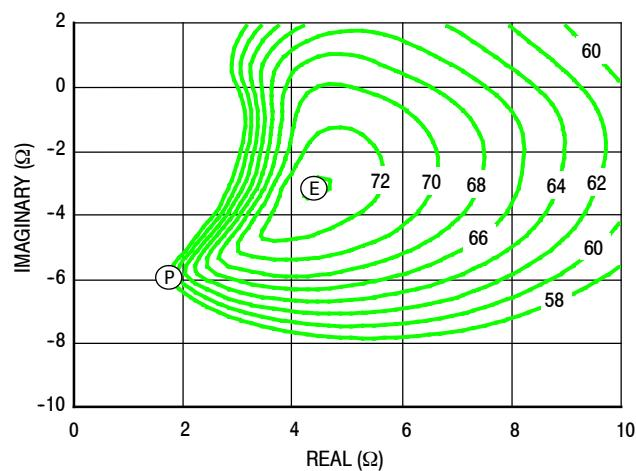
Figure 33. P3dB Load Pull Efficiency Contours (%)
