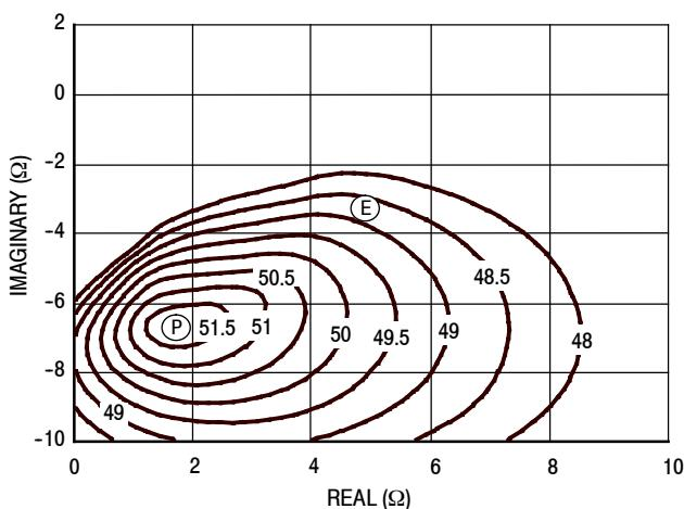
Figure 40. P3dB Load Pull Output Power Contours (dBm)
