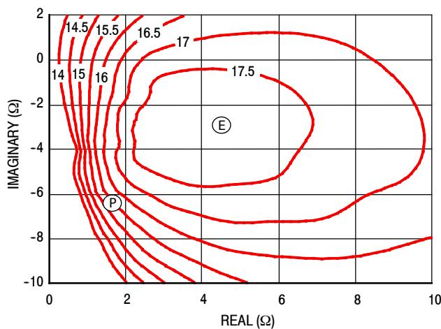
Figure 38. P1dB Load Pull Gain Contours (dB)
