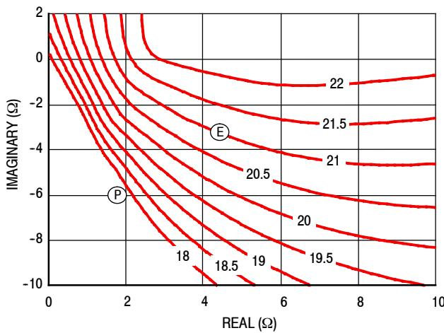
Figure 34. P3dB Load Pull Gain Contours (dB)
