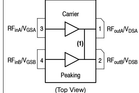
**Figure 1. Pin Connections**
