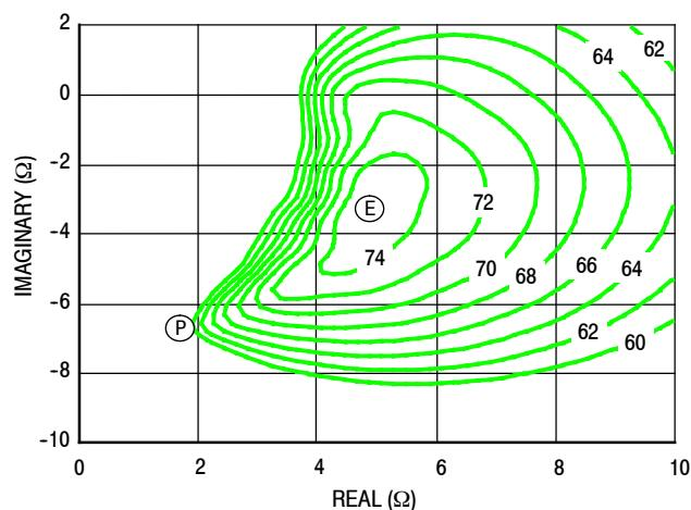
Figure 41. P3dB Load Pull Efficiency Contours (%)
