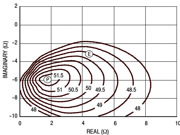
Figure 32. P3dB Load Pull Output Power Contours (dBm)
