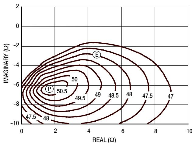
Figure 36. P1dB Load Pull Output Power Contours (dBm)
