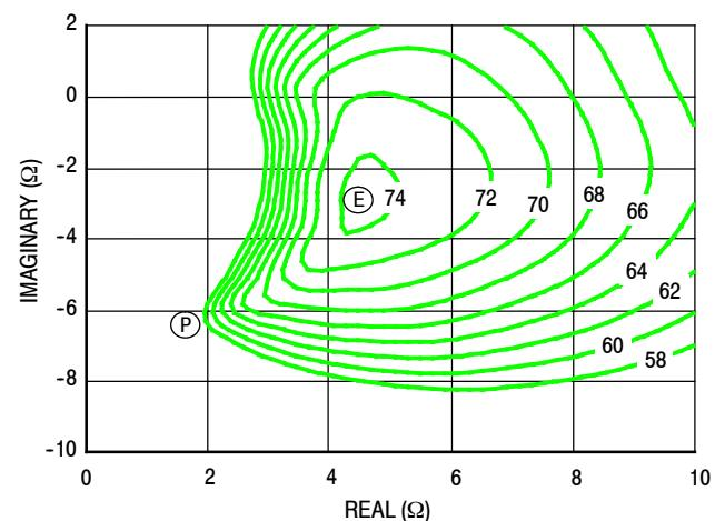
Figure 37. P1dB Load Pull Efficiency Contours (%)
