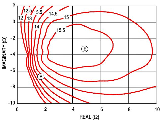
Figure 42. P3dB Load Pull Gain Contours (dB)
