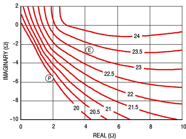
Figure 30. P1dB Load Pull Gain Contours (dB)
