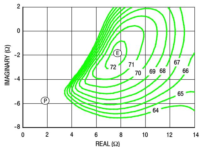
Figure 17. P1dB Load Pull Efficiency Contours (%)
