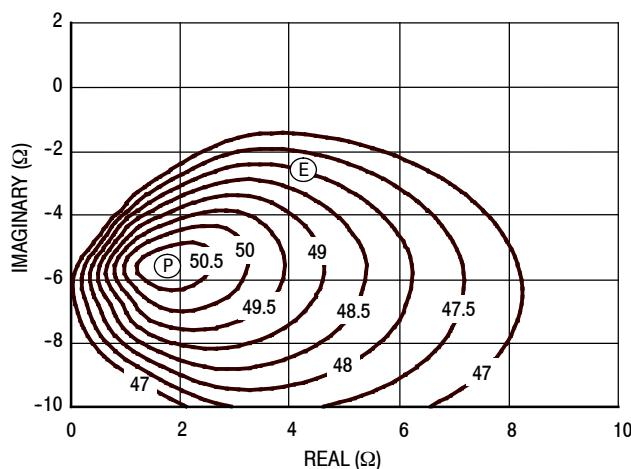
Figure 28. P1dB Load Pull Output Power Contours (dBm)
