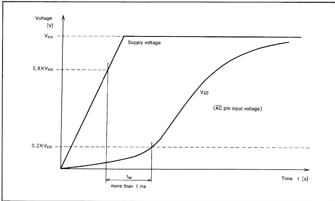
Fig. 16 Timing of power supplying to  $\overline{AC}$  pin
