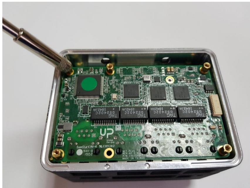
7. Place the bottom base on top of the NET Plus housing and tighten this with the M2.5\*4 screws which are reserved at first step.
