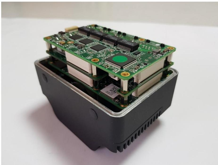
5. Place the NET Plus housing on the top of the main housing, checking the IO side, make sure the I/O is exactly matching the panel side.
