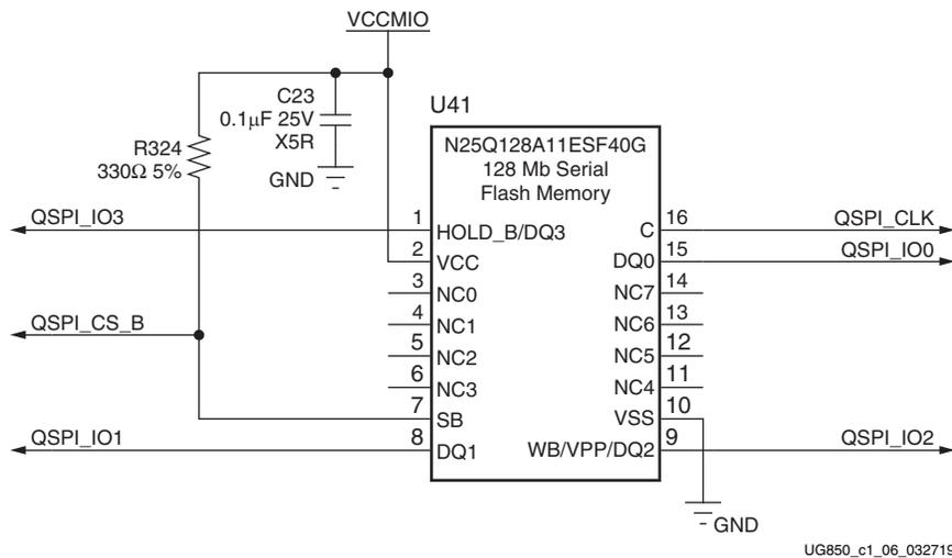
Figure 1-6: 128 Mb Quad-SPI Flash Memory (U41)
