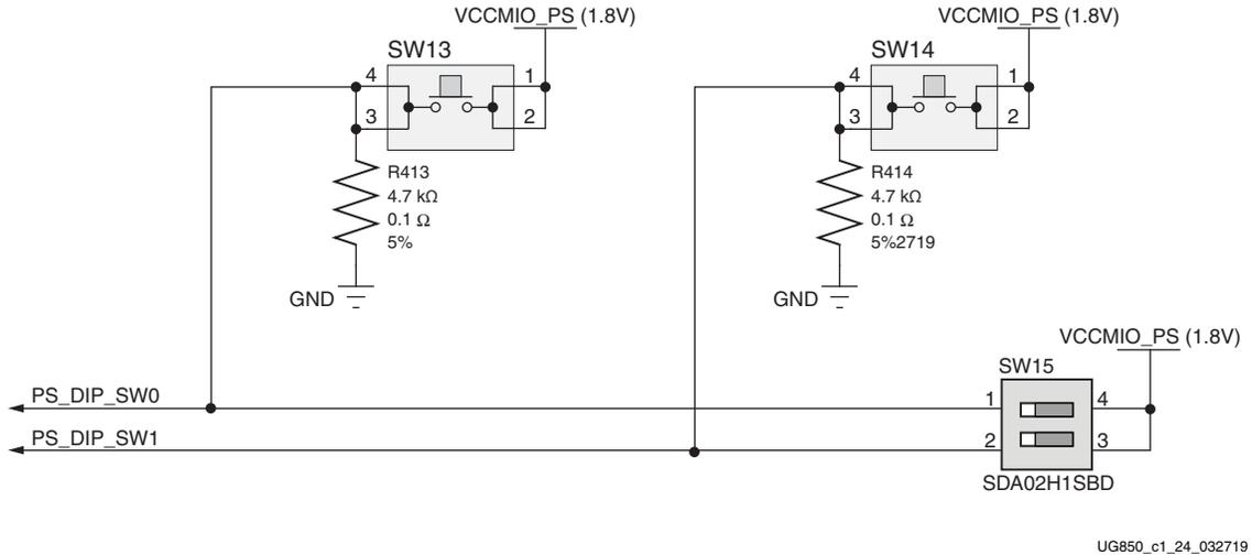
Figure 1-24: User PS Pushbutton and DIP Switch Circuit
