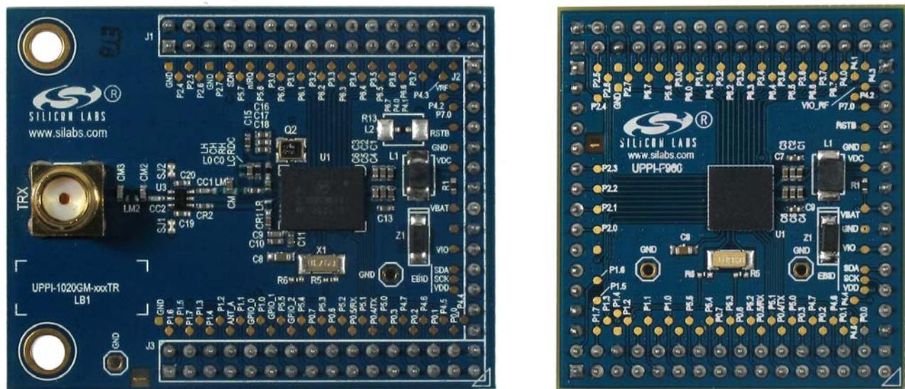
Figure 1. UPPI Cards with and without Radio
