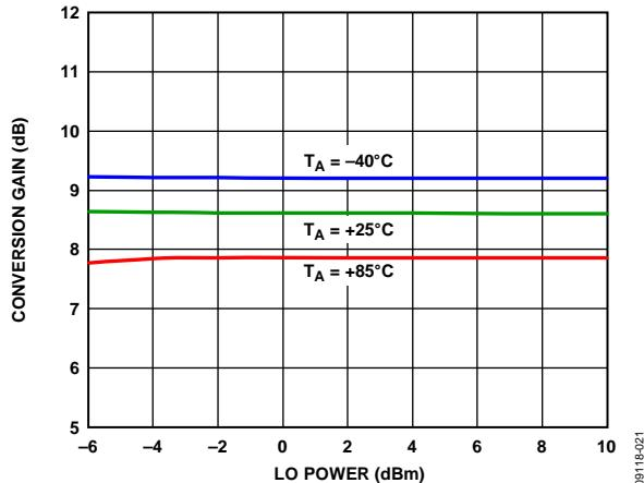
Figure 21. Power Conversion Gain vs. LO Power
