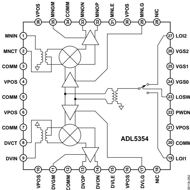
Figure 51. Simplified Schematic
