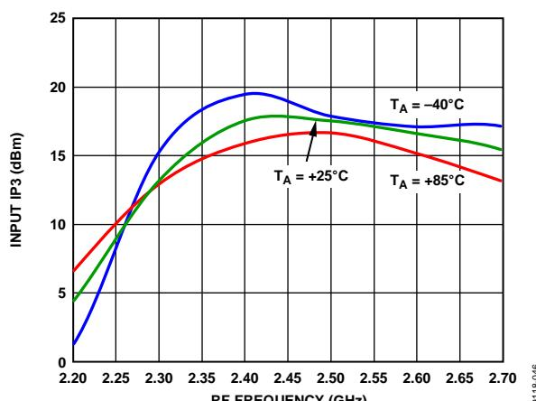
Figure 47. Input IP3 vs. RF Frequency at 3.3 V
