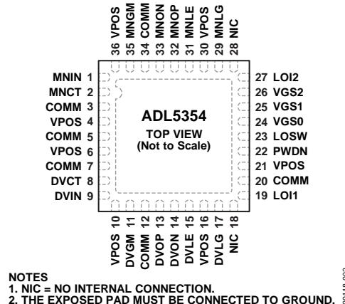
Figure 2. Pin Configuration
