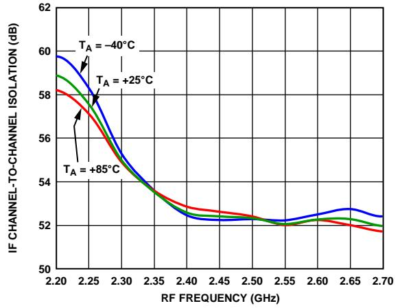
Figure 44. IF Channel-to-Channel Isolation vs. RF Frequency
