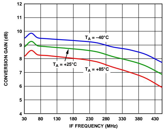
Figure 16. Power Conversion Gain vs. IF Frequency
