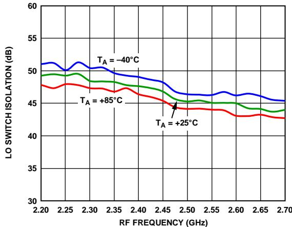
Figure 33. LO Switch Isolation vs. RF Frequency
