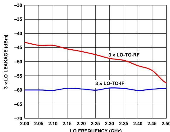
Figure 38. 3x LO Leakage vs. LO Frequency
