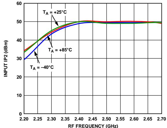
Figure 48. Input IP2 vs. RF Frequency at 3.3 V
