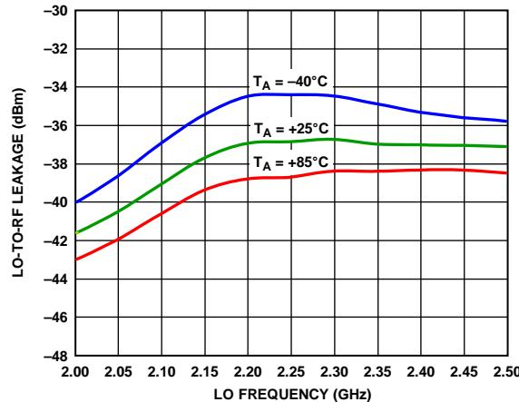
Figure 36. LO-to-RF Leaks vs. LO Frequency
