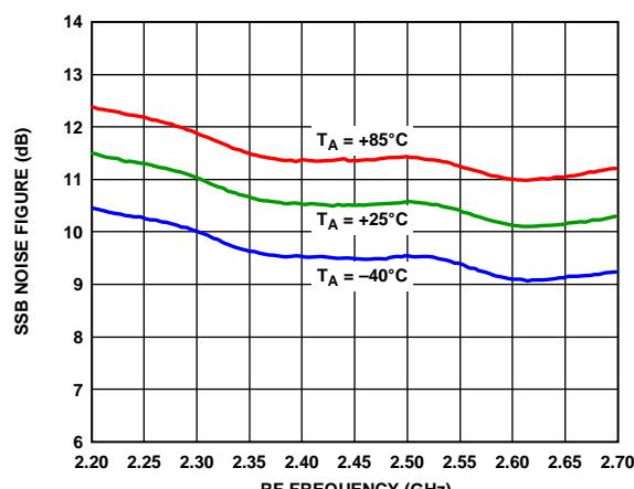
Figure 8. SSB Noise Figure vs. RF Frequency
