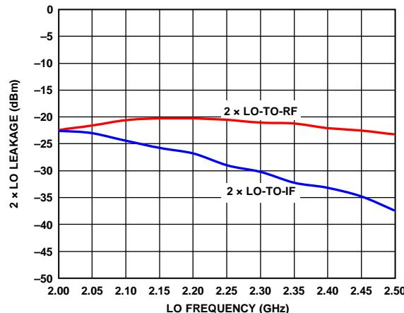
Figure 37. 2x LO Leakage vs. LO Frequency
