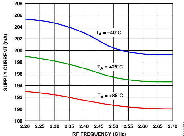
Figure 45. Supply Current vs. RF Frequency at 3.3 V
