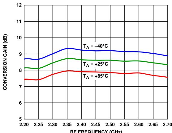
Figure 4. Power Conversion Gain vs. RF Frequency
