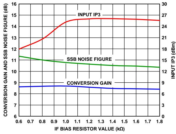
Figure 43. Power Conversion Gain, SSB Noise Figure, and Input IP3 vs. IF Bias Resistor Value
