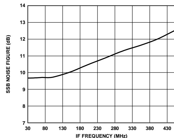
Figure 20. SSB Noise Figure vs. IF Frequency
