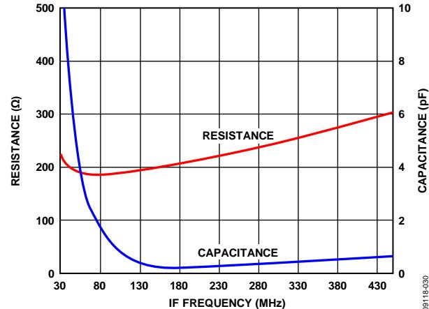
Figure 30. IF Output Impedance ( $R$  Parallel,  $C$  Equivalent)
