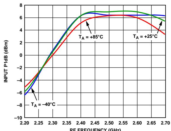
Figure 49. Input P1dB vs. RF Frequency at 3.3 V
