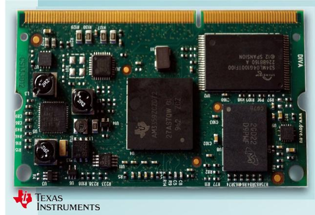
DIVA is a ready-to-use CPU module by DAVE Embedded Systems, based on Texas Instruments Cortex-A8 application processor from AM335x (Sitara) family.
