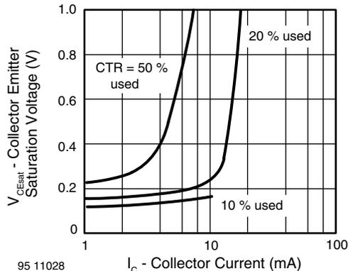
Fig. 10 - Collector Emitter Saturation Voltage vs. Collector Current
