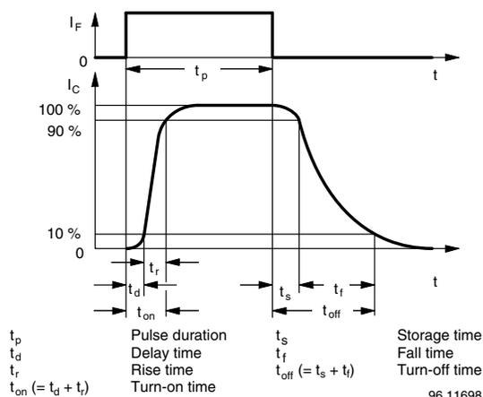
Fig. 3 - Switching Times
