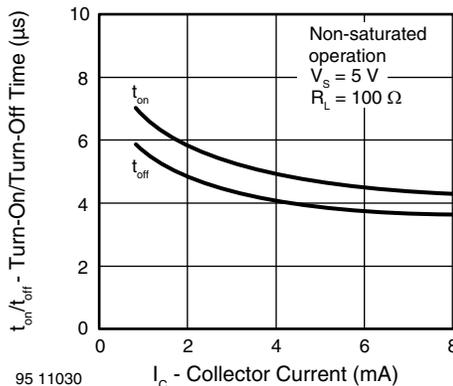
Fig. 13 - Turn-on/off Time vs. Collector Current
