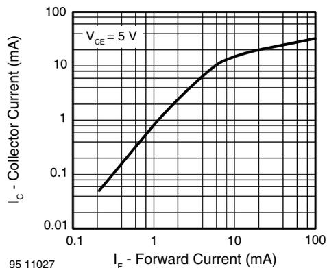
Fig. 8 - Collector Current vs. Forward Current
