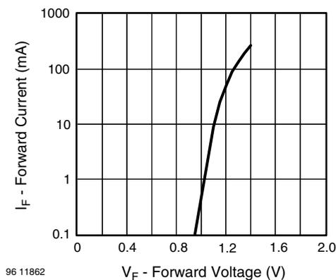
Fig. 5 - Forward Current vs. Forward Voltage
