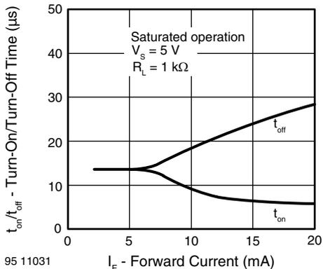
Fig. 12 - Turn-on/off Time vs. Forward Current
