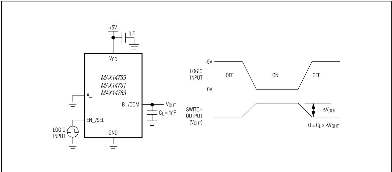
Figure 7. Charge Injection
