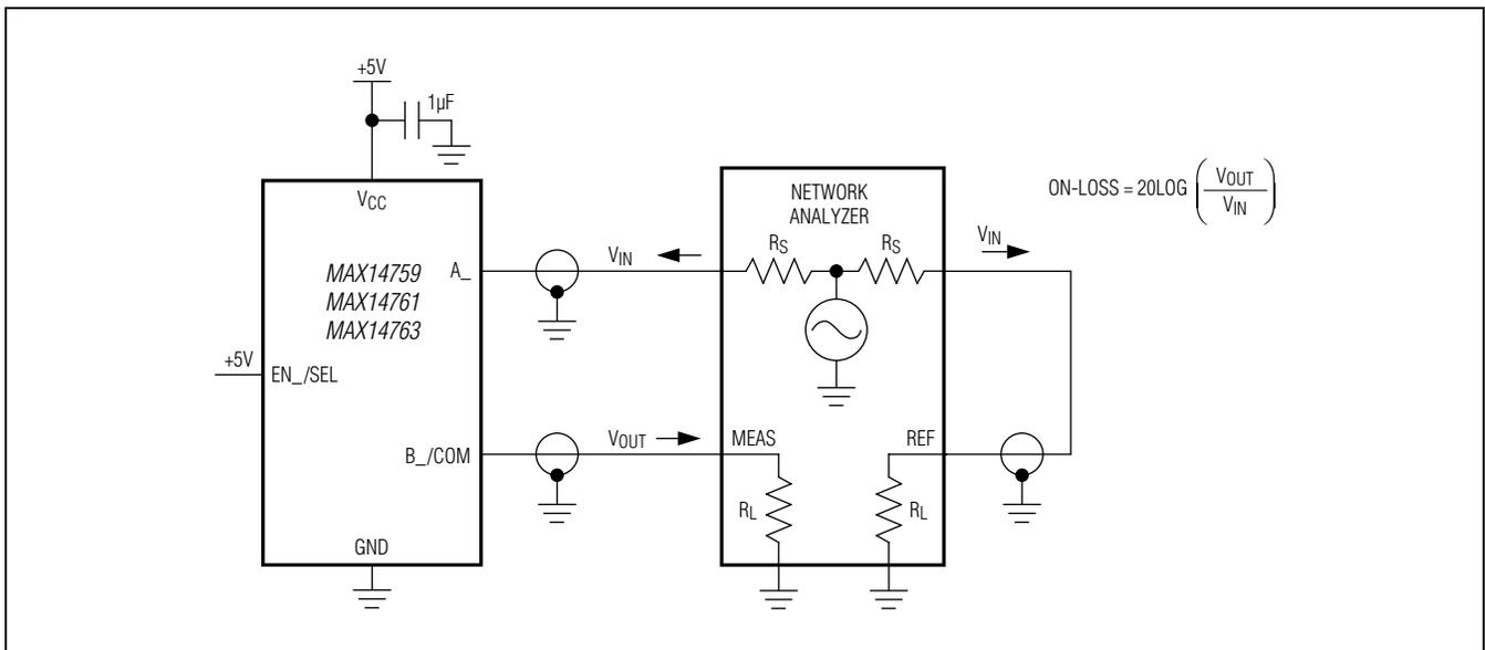
Figure 6. Insertion Loss
