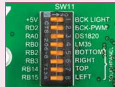
Figure 20-3: Enabled SW11.3 DIP switch
