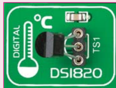
Figure 20-2: DS1820 correctly placed in socket
