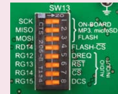
Figure 14-2: Enabling audio codec communication lines
