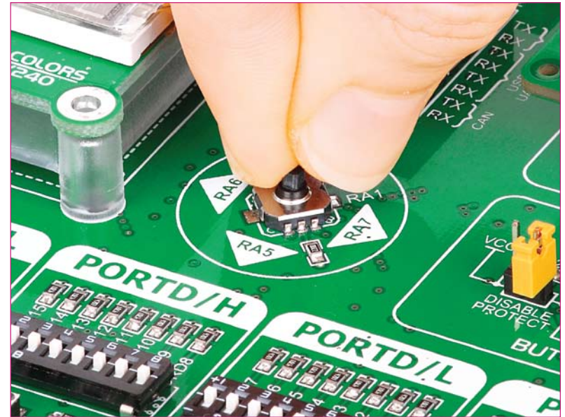
Figure 18-2: Navigation switch is an intuitive solution for browsing through on-screen menus.
