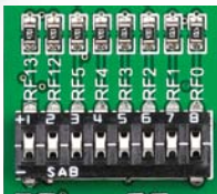
Figure 6-2: Tri-state DIP switch on PORTF
