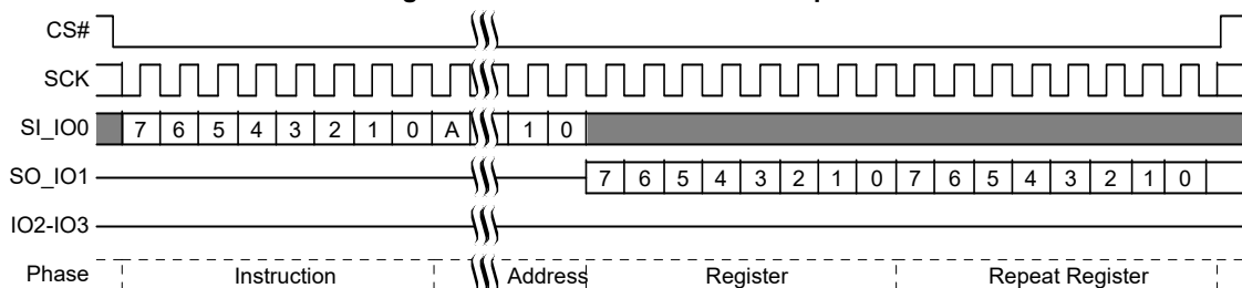
Figure 106. DYBRD Command Sequence
