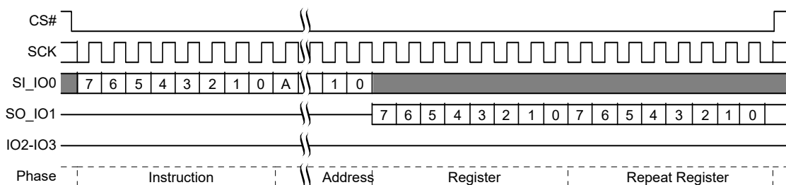
Figure 110. PPB Read Command Sequence
