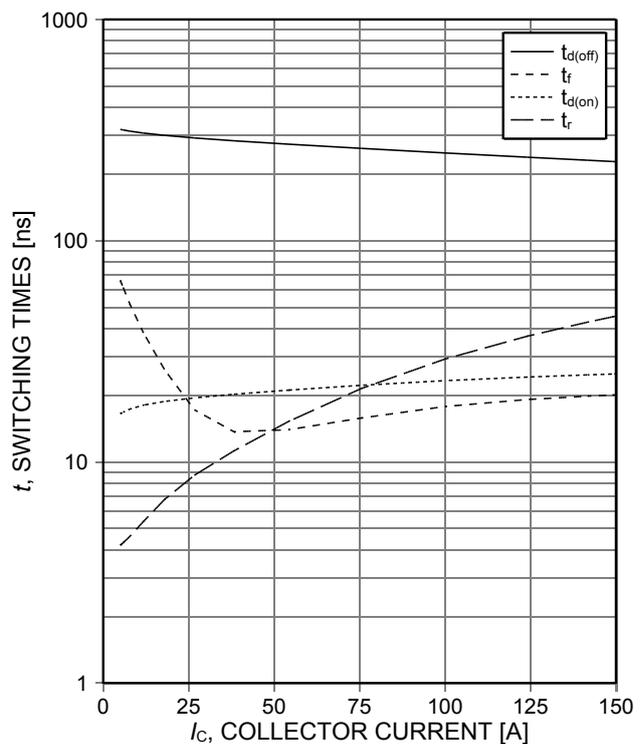
Figure 8. Typical switching times as a function of collector current (inductive load,  $T_{vj}=150^{\circ}\text{C}$ ,  $V_{CE}=400\text{V}$ ,  $V_{GE}=0/15\text{V}$ ,  $R_{G(on)}=12\Omega$ ,  $R_{G(off)}=20\Omega$ , dynamic test circuit in Figure E)
