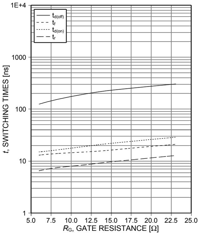
Figure 9. **Typical switching times as a function of gate resistance**
