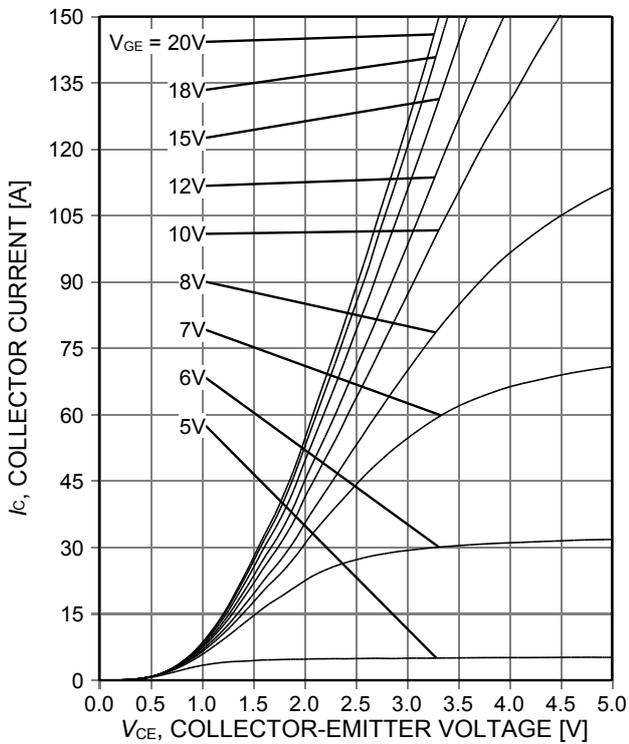
Figure 5. Typical output characteristic ( $T_{vj}=175^{\circ}\text{C}$ )
