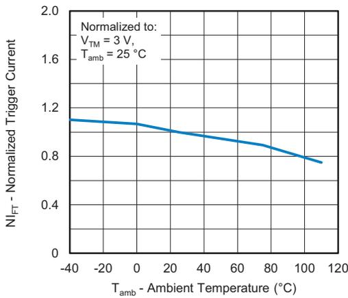
Fig. 4 - Normalized Trigger Current vs. Ambient Temperature
