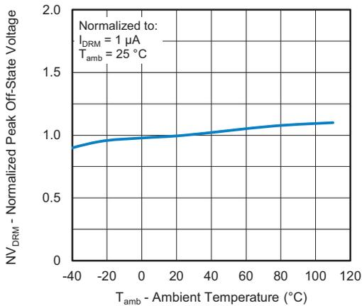
Fig. 10 - Normalized Peak Off-State Voltage vs. Ambient Temperature
