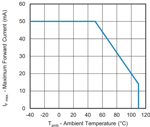
Fig. 1 - Maximum Forward Current vs. Ambient Temperature
