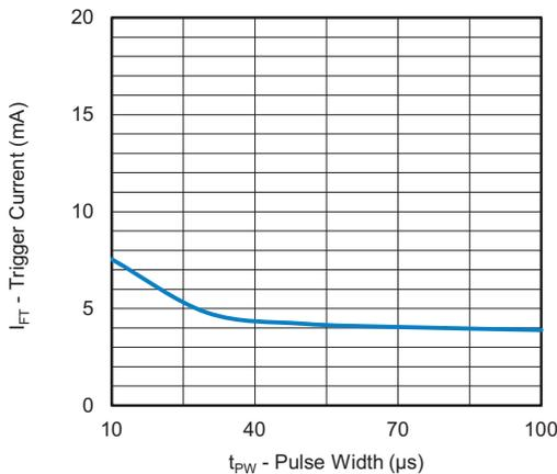
Fig. 5 - Trigger Current vs. Pulse Width
