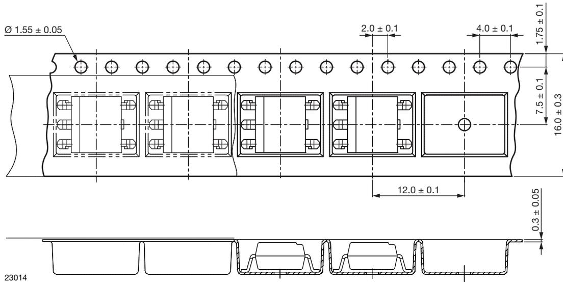
Fig. 16 - Tape and Reel Packaging (1000 pieces on reel)
