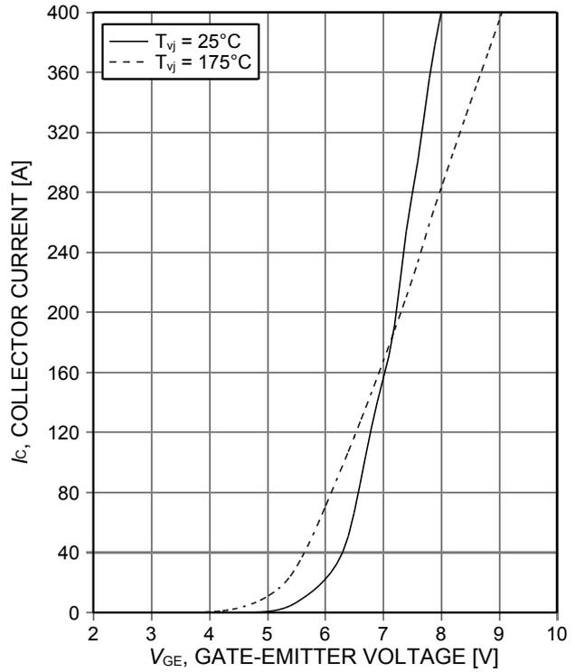
Figure 6. **Typical transfer characteristic**
